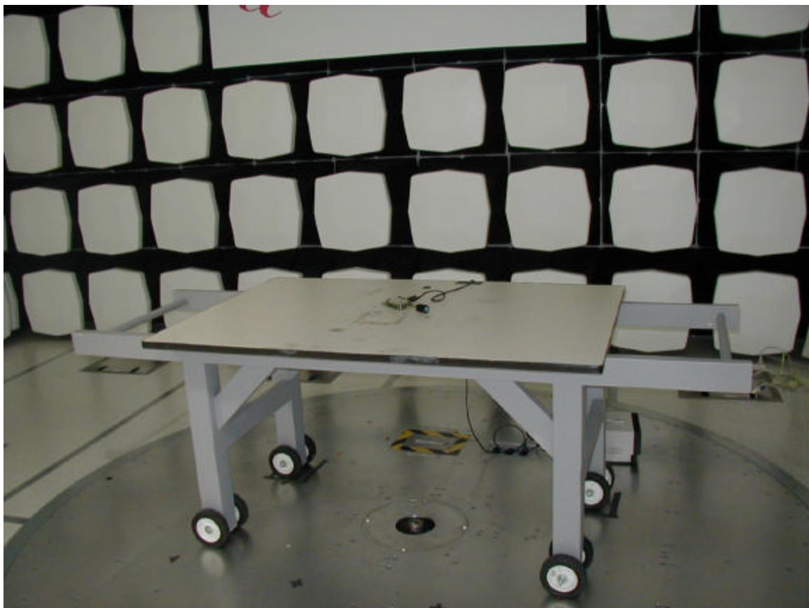
Radiate Emissions Test Configuration Photographs
