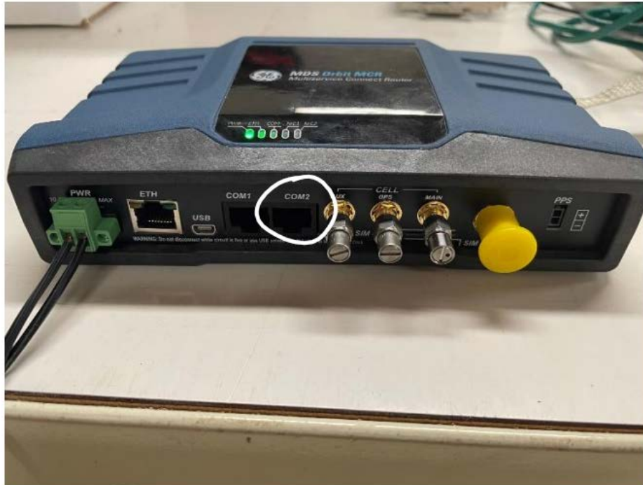
Figure 7: COM2 CLI (Command Line Interface) port for RCL220 inside of the Orbit MCR Host
