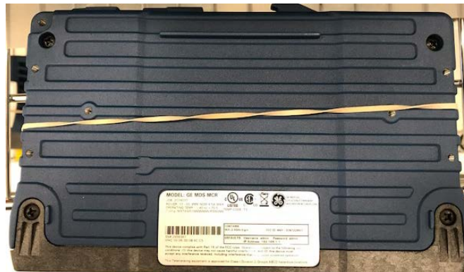
Figure 9: Location of label detailed in Figure 8, placed on the underside of the Orbit MCR
