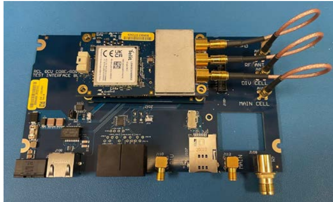
Figure 8: OCR220 Module Installed on test fixture
