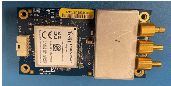
Figure 2: OCR220 Radio PCBA
