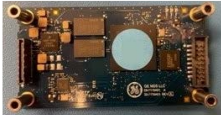
Figure 3: OCR220 Processor PCBA
