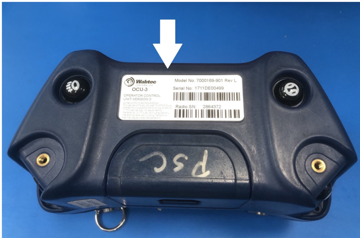
Figure 9: Location of label detailed in Figure 8, placed on the underside of the Wabtec OCU
