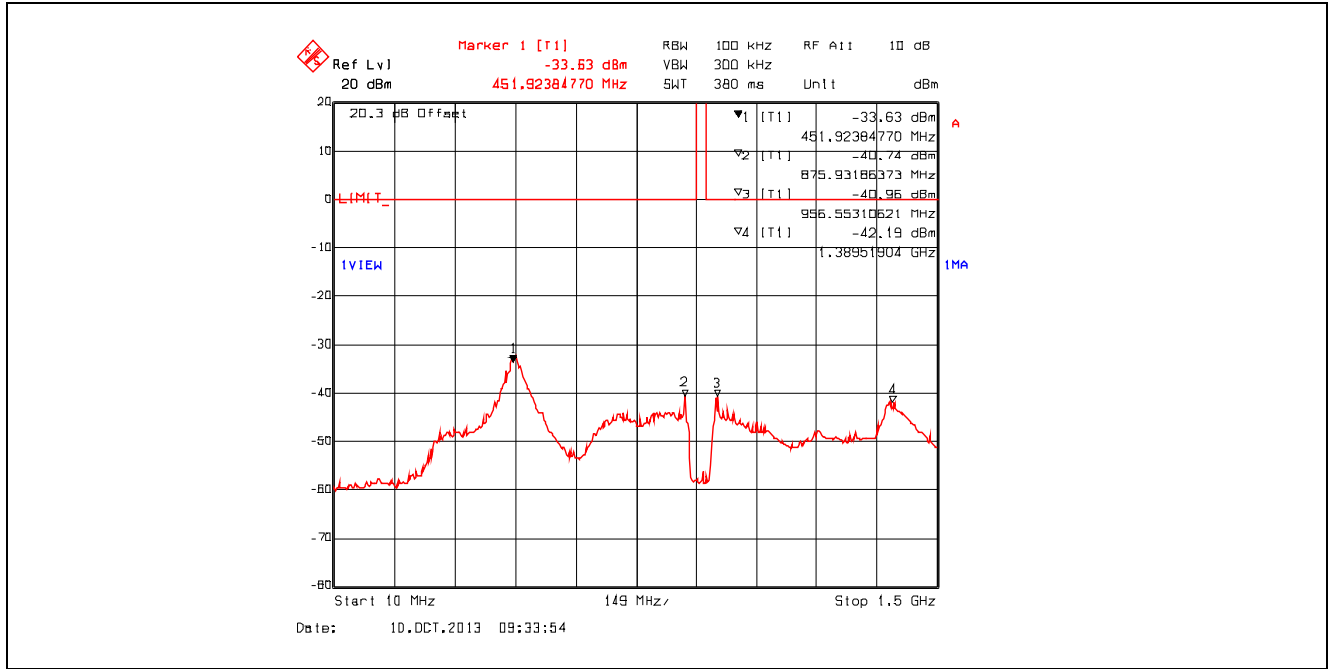
Plot 5.3.4.2.3. Conducted Spurious Emissions, High Power, 915.000 MHz, 10 MHz - 1.5 GHz
