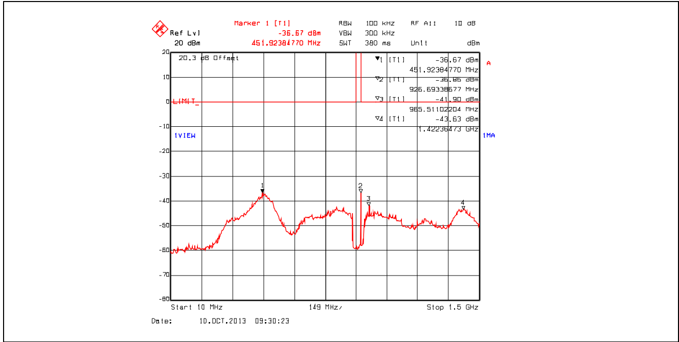
Plot 5.3.4.2.5. Conducted Spurious Emissions, High Power, 926.685 MHz, 10 MHz - 1.5 GHz
