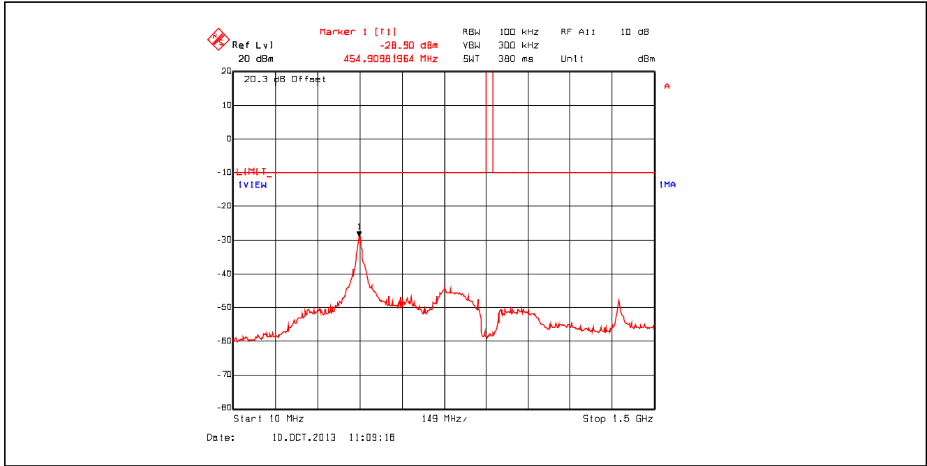
Plot 5.3.4.2.9. Conducted Spurious Emissions, Low Power, 915.000 MHz, 10 MHz - 1.5 GHz
