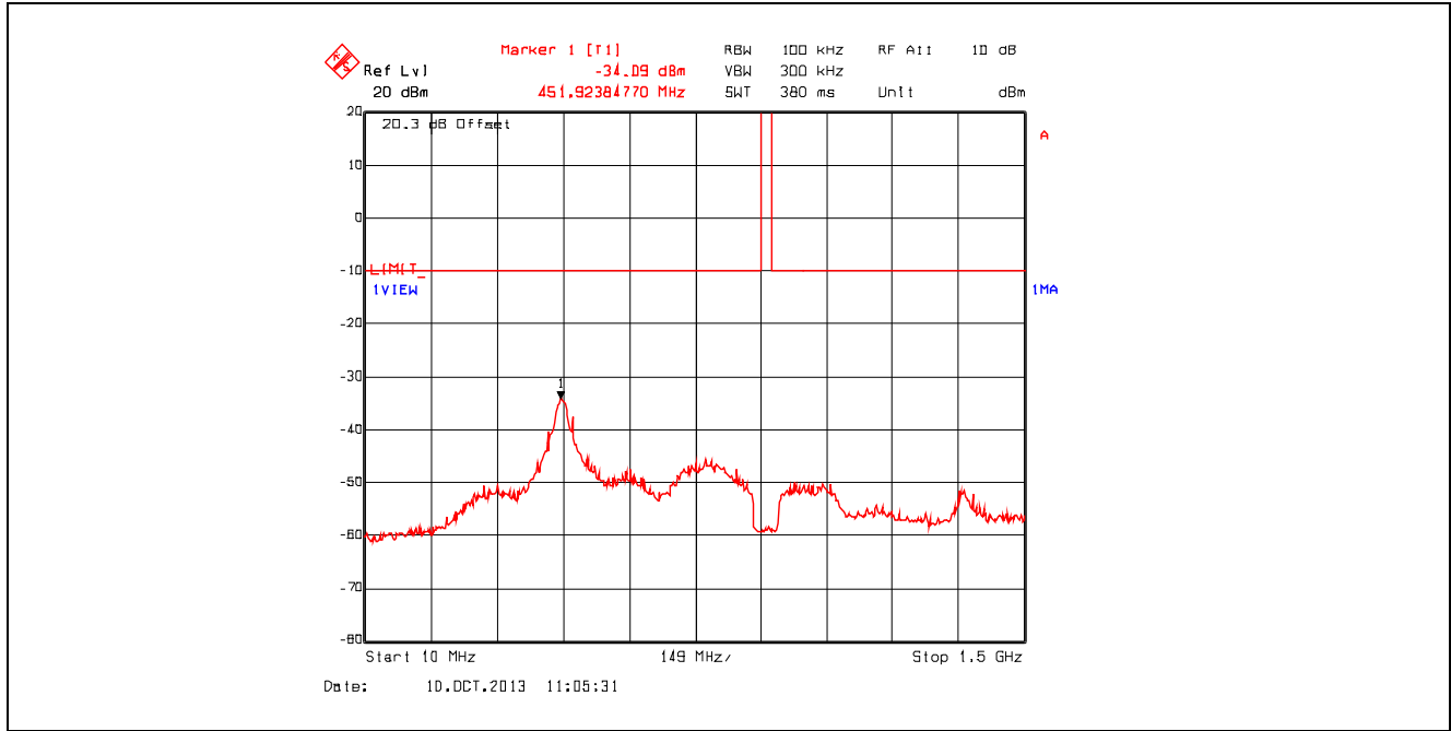
Plot 5.3.4.2.7. Conducted Spurious Emissions, Low Power, 903.315 MHz, 10 MHz - 1.5 GHz
