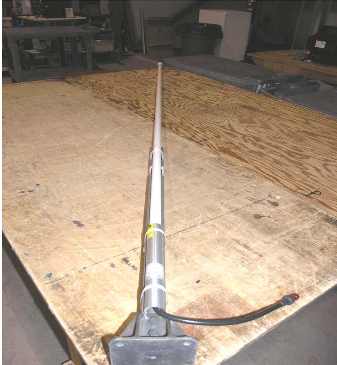
(9.15 dBi Gain Omni Directional Antenna)
