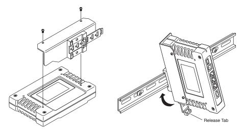
Step 1: Attach the bracket using the the two screws provided. (Attach to the end opposite the connectors.)
