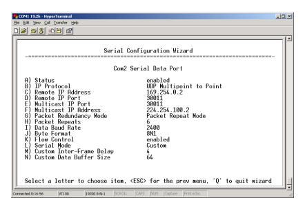
Figure 2-38. Remote Radio Serial Port Configuration
