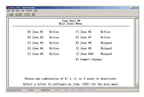
Figure 2-27. Skip Zone Options Submenu—GE MDS iNET Only ("Commit changes" displayed only on Access Point radios)
