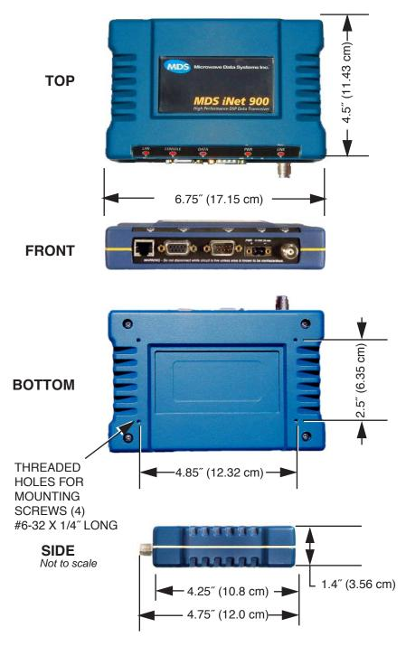
**Figure 4-2. Transceiver Dimensions**
