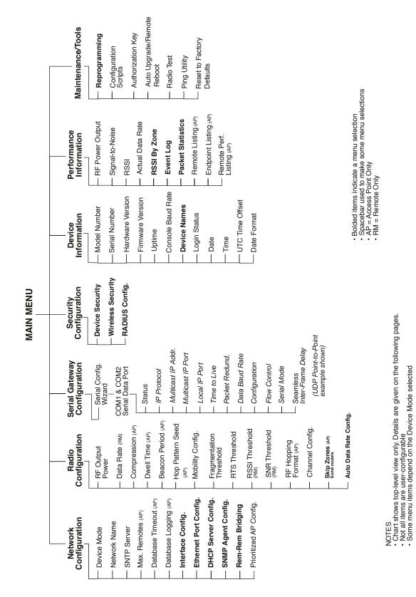
Figure 2-1. Embedded Management System—Top-level Flowchart
