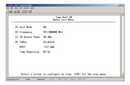
Figure 2-69. Radio Test Menu Shown with Test Mode set to ON
