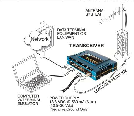
Figure 4-1. Typical Installation with a Tower-Mounted Antenna (Connect user data equipment to any compatible LAN or COM Port)
