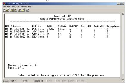
Figure 2-60. Remote Performance Listing Menu for iNET AP (iNET-II will show RxRate as 512 kbps or 1024 kbps)
