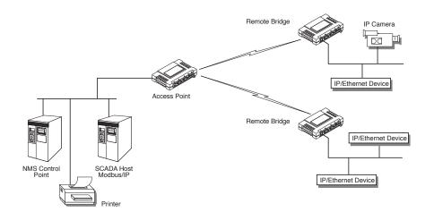
Figure 1-7. Extended-Range LAN with Mixed Applications
