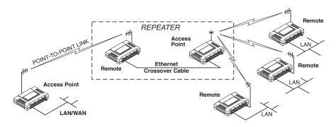
Figure 1-8. Typical LAN with a Repeater Link
