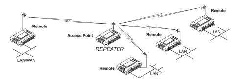
Figure 1-9. Typical network with store-and-forward repeater
