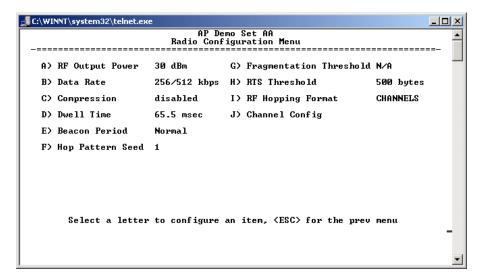
Figure 2-24. Radio Configuration Menu (From Access Point Unit)
