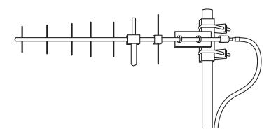
Figure 4-6. Typical Yagi Antenna (mounted to mast)
