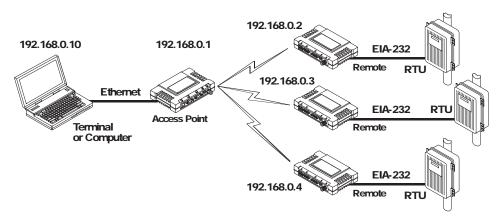
Figure 2-37. Point-to-Multipoint Serial-to-Serial Application Diagram
