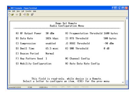
Figure 2-25. Radio Configuration Menu (From Remote Unit)
