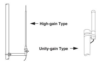
Figure 4-5. Typical Omnidirectional Antennas
