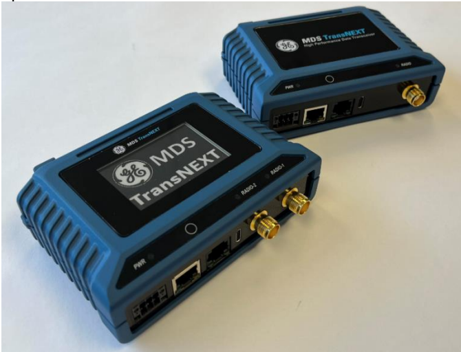
Figure 1. GE MDS TransNEXT Transceiver. Dual transceiver version (left) and single transceiver (right).
