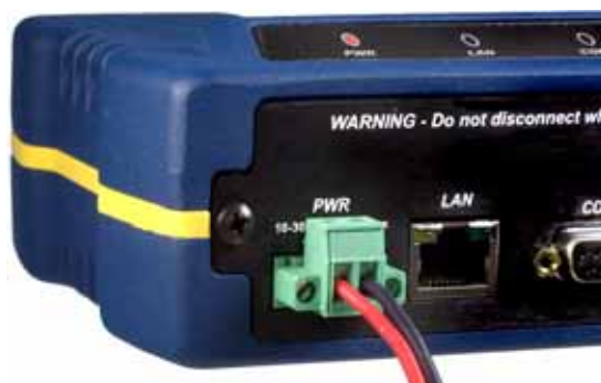
Figure 2-2. Power Connector (Polarity: Left +, Right –)
