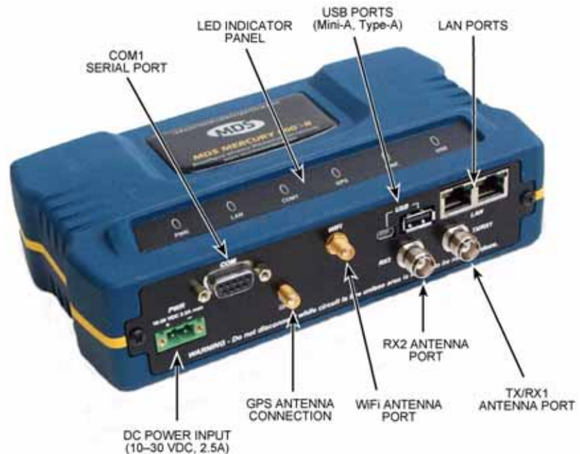
Figure 2-4. Option 1 Set Transceiver Interface Connectors
