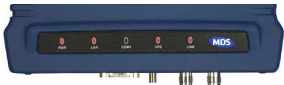
Figure 2-5. LED Indicator Panel
