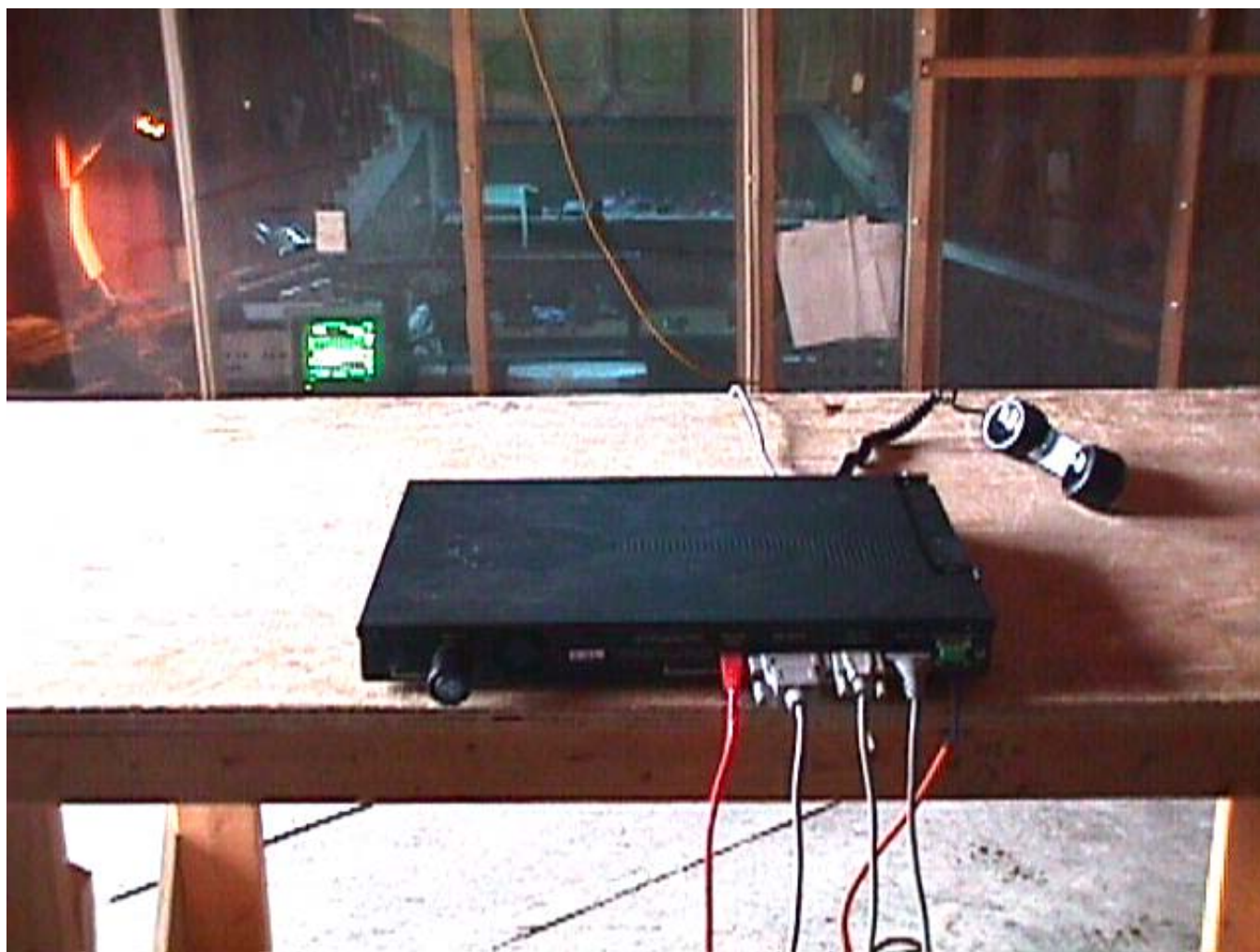
Transmitter Radiated Emissions Test Setup (at 3 meters distance)
