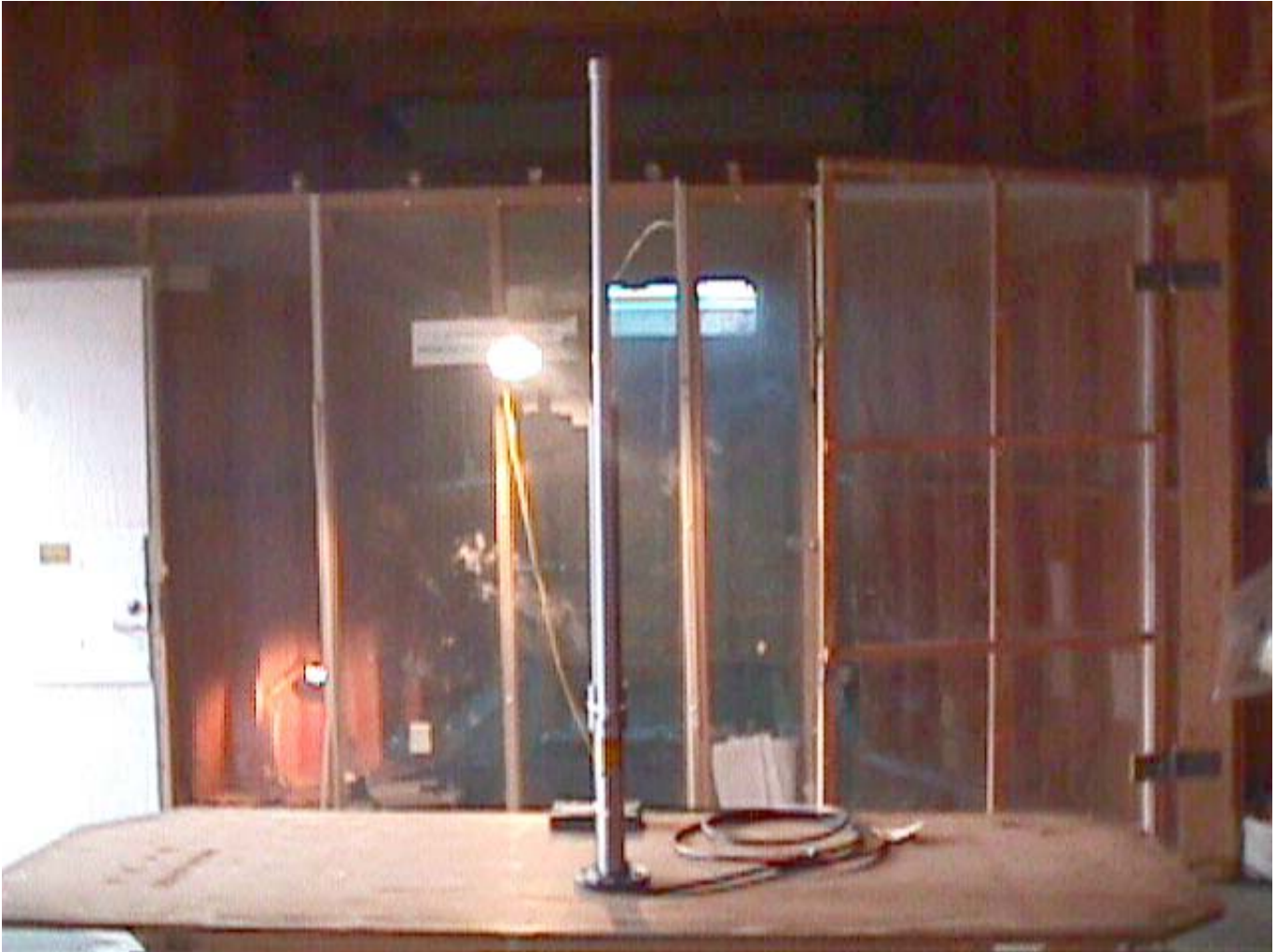
EUT with MDS ClearWave Omni-directional Base Station Antenna
