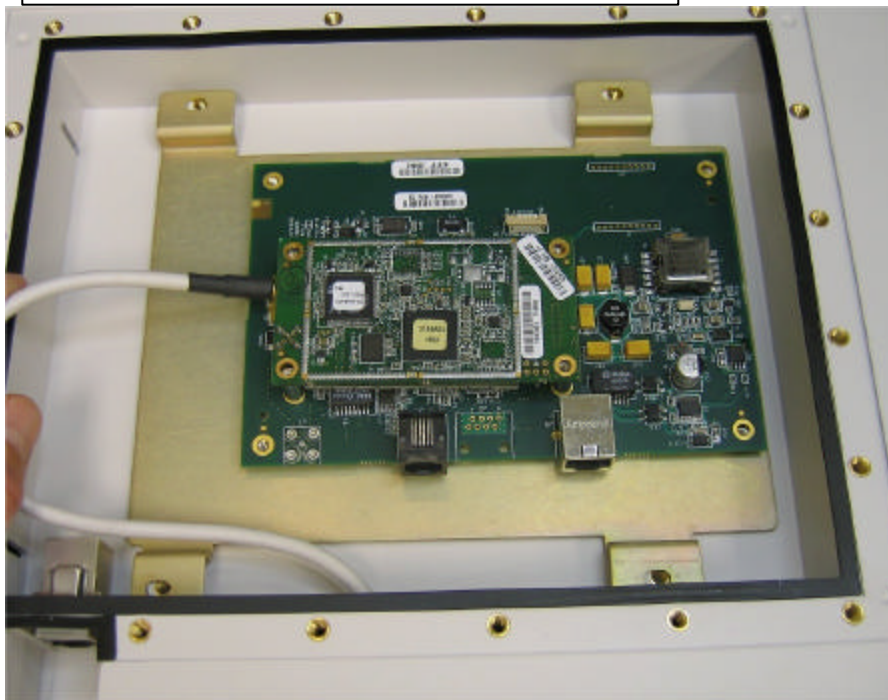
EL806 installed onto motherboard inside Panel antenna
