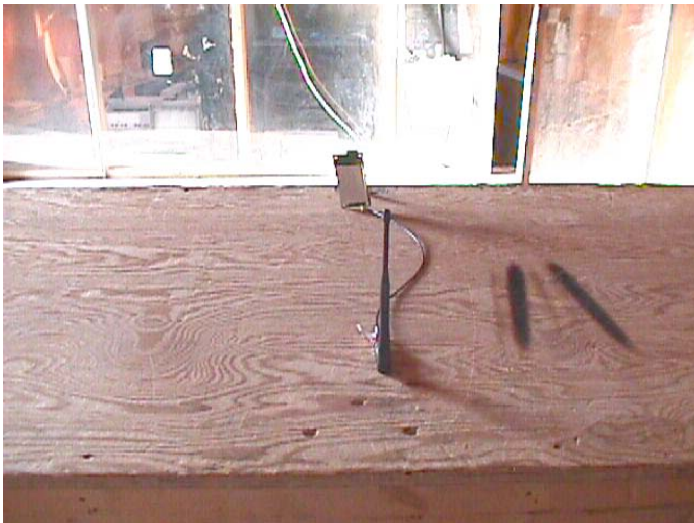
EUT with MDS ClearWave 1/2 Wave Dipole Antenna
