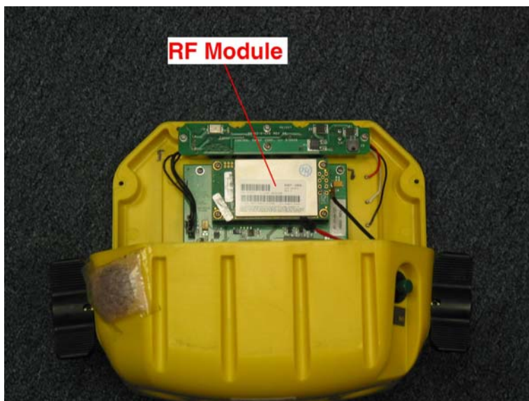
RF Module Location on Inside Back of Device
