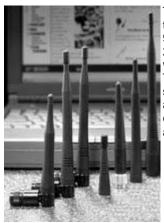
The MAXRAD portable antennas are designed to cover the band of frequencies from 902-928 MHz ISM, 1710-1990 MHz PCS, 2400 to 2483.5 MHz ISM and 5725-5825 MHz ISM with a VSWR of less than 1.5:1 at resonance. Their rugged, flexible design makes them suitable for use in a wide variety of applications, including office LAN environments, factory floors, remote telemetry and other harsh environments.
