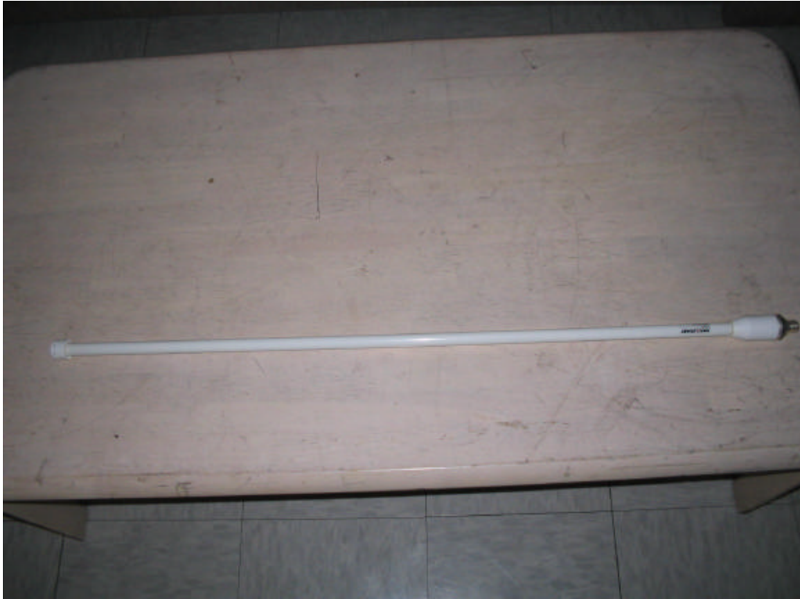
2.4GHz Omni-Directional antenna, Manufacture: MAXRAD (M/N: MFB24010) 10dBi gain
