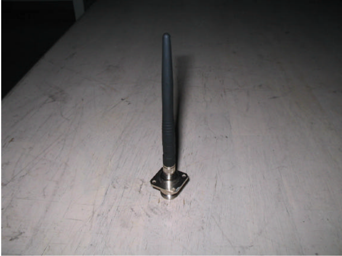
2.4GHz Stub antenna, Manufacture: MAXRAD (M/N: MHWS2400MSMA) 2 dBi gain
