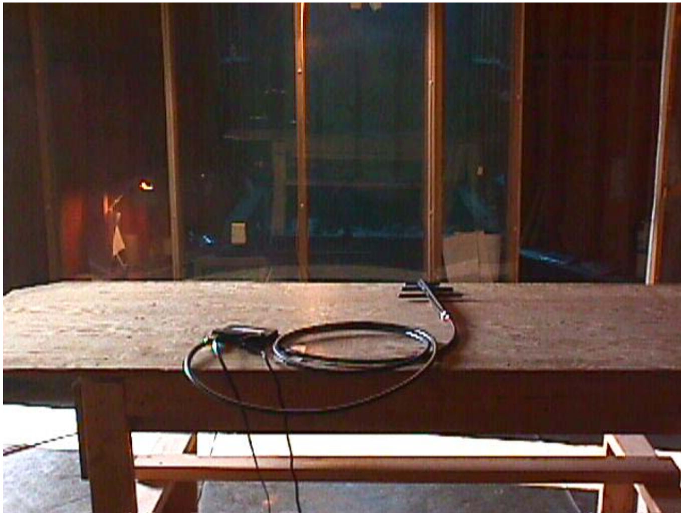
Test Configuration 4: Plastic Enclosure with MDS ClearWave Yagi Antenna (Rear View)
