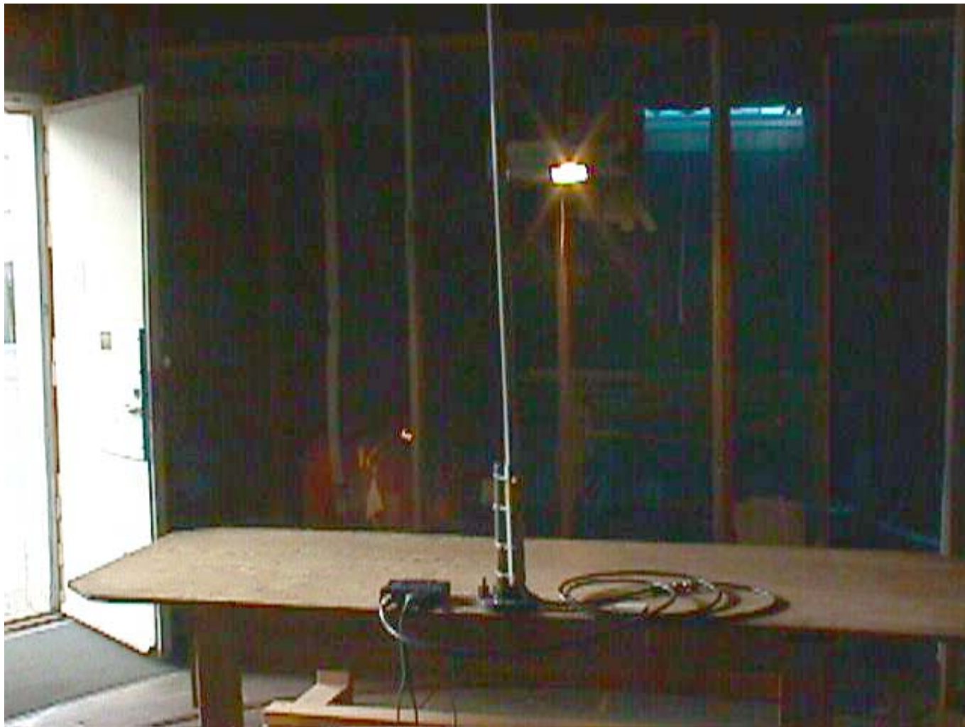
Test Configuration 1: Metallic Enclosure with Maxrad 900 MHz Omnis-MFB Antenna (Rear View)
