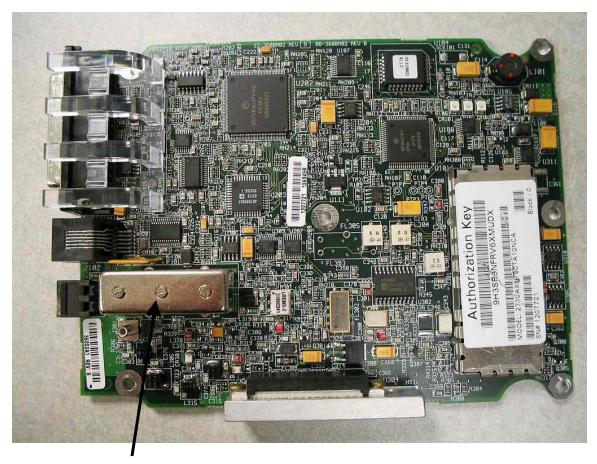
This is as pre-assembled tunable component, by the manufacture, and trying to open it will cause permanent damage.
