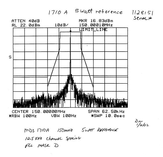
Plot # 14 Emission Mask D Carrier Frequency: 150 MHz Channel Spacing: 12.5 kHz Power: 5 W Comment: Test results provided by the manufacturer, Microwave Data Systems Inc.
