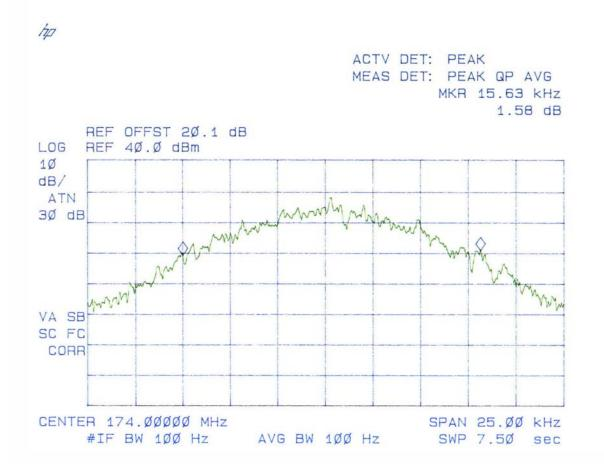
Plot # 7 Emission Mask B Carrier Frequency: 150 MHz Channel Spacing: 25 kHz Power: 5 W
