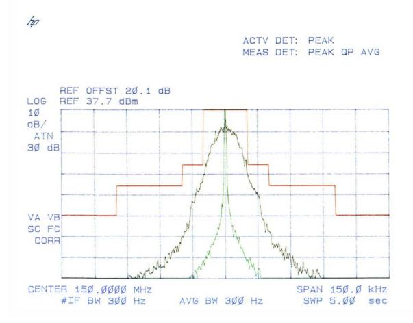
Plot # 8 Emission Mask B Carrier Frequency: 162 MHz Channel Spacing: 25 kHz Power: 5 W
