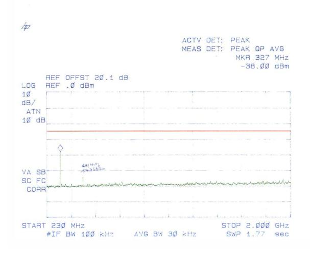
Plot #29 Spurious Emissions at Antenna Terminals Carrier Frequency: 174 MHz Channel Spacing: 12.5 kHz Power: 0.1 W
