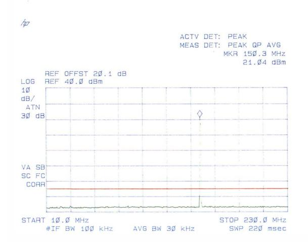
Plot # 22 Spurious Emissions at Antenna Terminals Carrier Frequency: 150 MHz Channel Spacing: 12.5 kHz Power: 0.1 W
