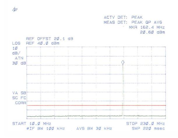
Plot # 26 Spurious Emissions at Antenna Terminals Carrier Frequency: 162 MHz Channel Spacing: 12.5 kHz Power: 0.1 W
