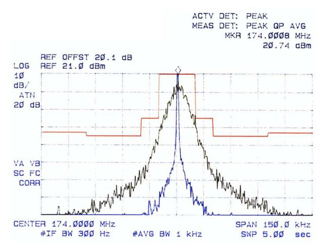
Plot # 13 Emission Mask D Carrier Frequency: 150 MHz Channel Spacing: 12.5 kHz Power: 5 W Comment: Test results provided by the manufacturer, Microwave Data Systems Inc.
