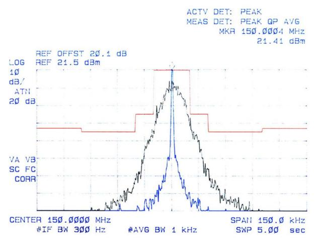
Plot # 11 Emission Mask B Carrier Frequency: 162 MHz Channel Spacing: 25 kHz Power: 100 mW
