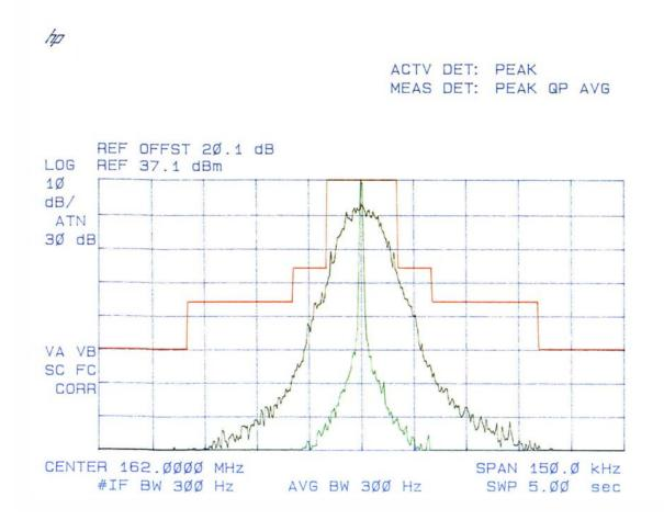
Plot # 9 Emission Mask B Carrier Frequency: 174 MHz Channel Spacing: 25 kHz Power: 5 W
