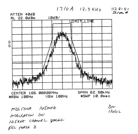
Plot # 17 Emission Mask D Carrier Frequency: 165 MHz Channel Spacing: 12.5 kHz Power: 5 W Comment: Test results provided by the manufacturer, Microwave Data Systems Inc.
