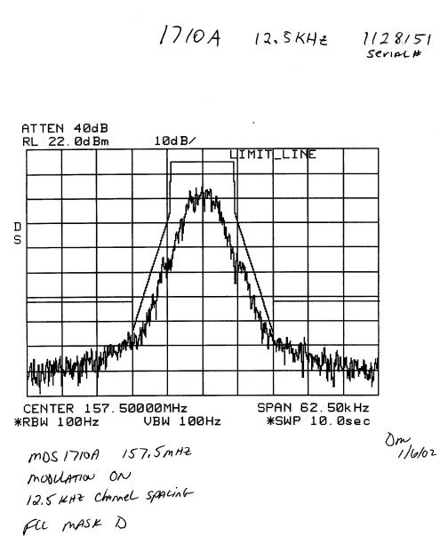
Plot # 16 Emission Mask D Carrier Frequency: 165 MHz Channel Spacing: 12.5 kHz Power: 5 W Comment: Test results provided by the manufacturer, Microwave Data Systems Inc.
