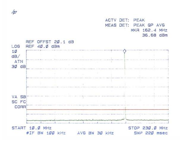
Plot # 28 Spurious Emissions at Antenna Terminals Carrier Frequency: 162 MHz Channel Spacing: 12.5 kHz Power: 5 W
