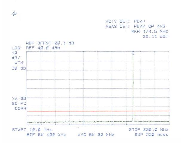
Plot # 32 Spurious Emissions at Antenna Terminals Carrier Frequency: 174 MHz Channel Spacing: 12.5 kHz Power: 5 W
