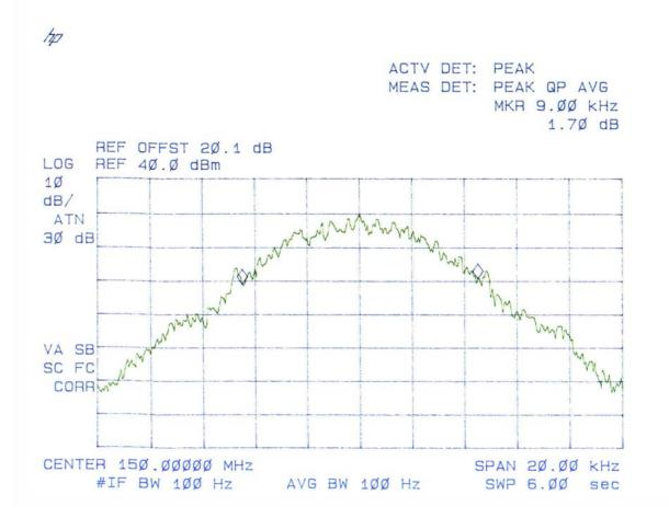
Plot # 2 99 % Occupied Bandwidth Carrier Frequency: 162 MHz Channel Spacing: 12.5 kHz Power: 5 W
