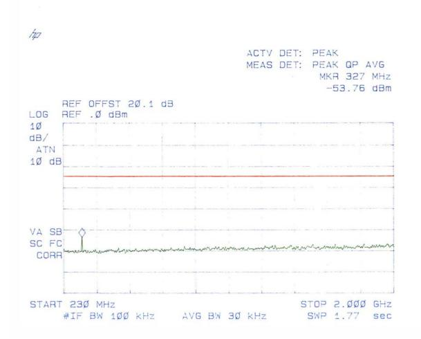
Plot # 27 Spurious Emissions at Antenna Terminals Carrier Frequency: 162 MHz Channel Spacing: 12.5 kHz Power: 5 W
