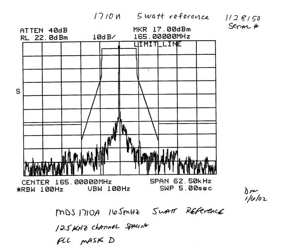
Plot # 18 Emission Mask D Carrier Frequency: 165 MHz Channel Spacing: 12.5 kHz Power: 5 W Comment: Test results provided by the manufacturer, Microwave Data Systems Inc.
