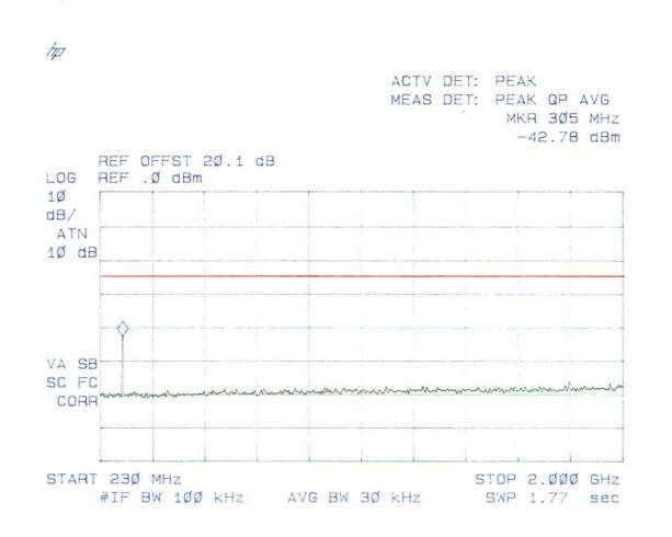
Plot # 23 Spurious Emissions at Antenna Terminals Carrier Frequency: 150 MHz Channel Spacing: 12.5 kHz Power: 5 W
