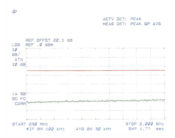
Plot # 31 Spurious Emissions at Antenna Terminals Carrier Frequency: 174 MHz Channel Spacing: 12.5 kHz Power: 5 W
