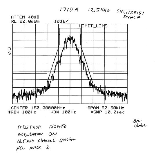
Plot # 15 Emission Mask D Carrier Frequency: 157.5 MHz Channel Spacing: 12.5 kHz Power: 5 W Comment: Test results provided by the manufacturer, Microwave Data Systems Inc.
