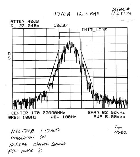
Plot # 20 Emission Mask D Carrier Frequency: 174 MHz Channel Spacing: 12.5 kHz Power: 5 W Comment: Test results provided by the manufacturer, Microwave Data Systems Inc.
