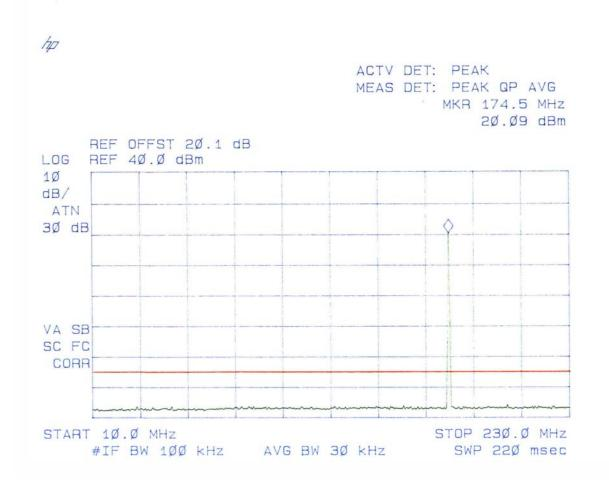
Plot # 30 Spurious Emissions at Antenna Terminals Carrier Frequency: 174 MHz Channel Spacing: 12.5 kHz Power: 0.1 W
