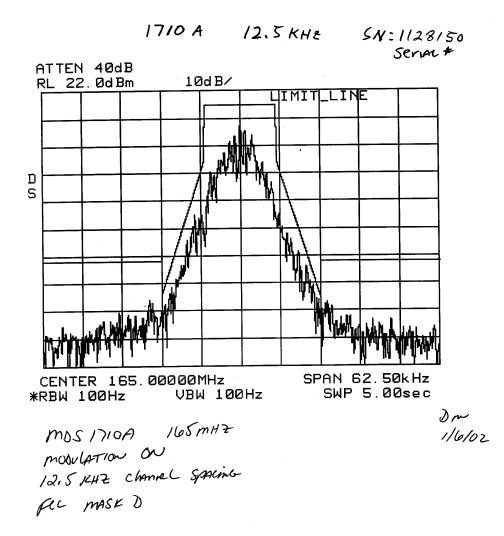
Plot # 19 Emission Mask D Carrier Frequency: 170 MHz Channel Spacing: 12.5 kHz Power: 5 W Comment: Test results provided by the manufacturer, Microwave Data Systems Inc.
