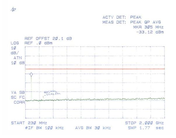
Plot #25 Spurious Emissions at Antenna Terminals Carrier Frequency: 162 MHz Channel Spacing: 12.5 kHz Power: 0.1 W
