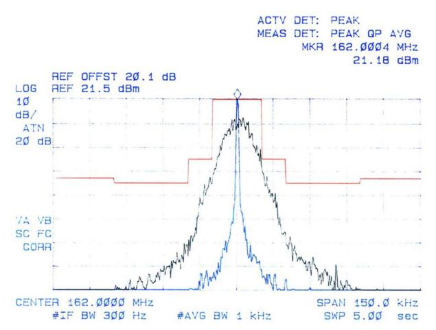
Plot # 12 Emission Mask B Carrier Frequency: 174 MHz Channel Spacing: 25 kHz Power: 100 mW
