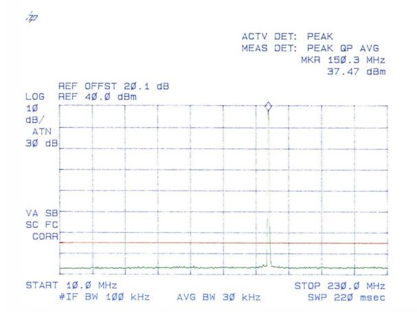
Plot # 24 Spurious Emissions at Antenna Terminals Carrier Frequency: 150 MHz Channel Spacing: 12.5 kHz Power: 5 W
