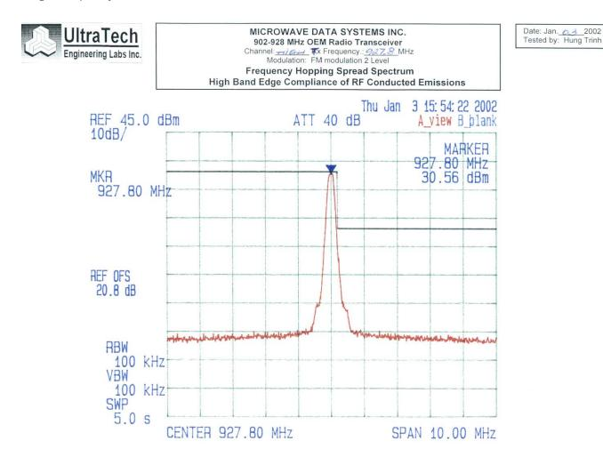
Plot # 14 Band-Edge Spurious Emissions at Antenna Terminals High End of Frequency Band Pseudorandom Channel Hopping Mode
