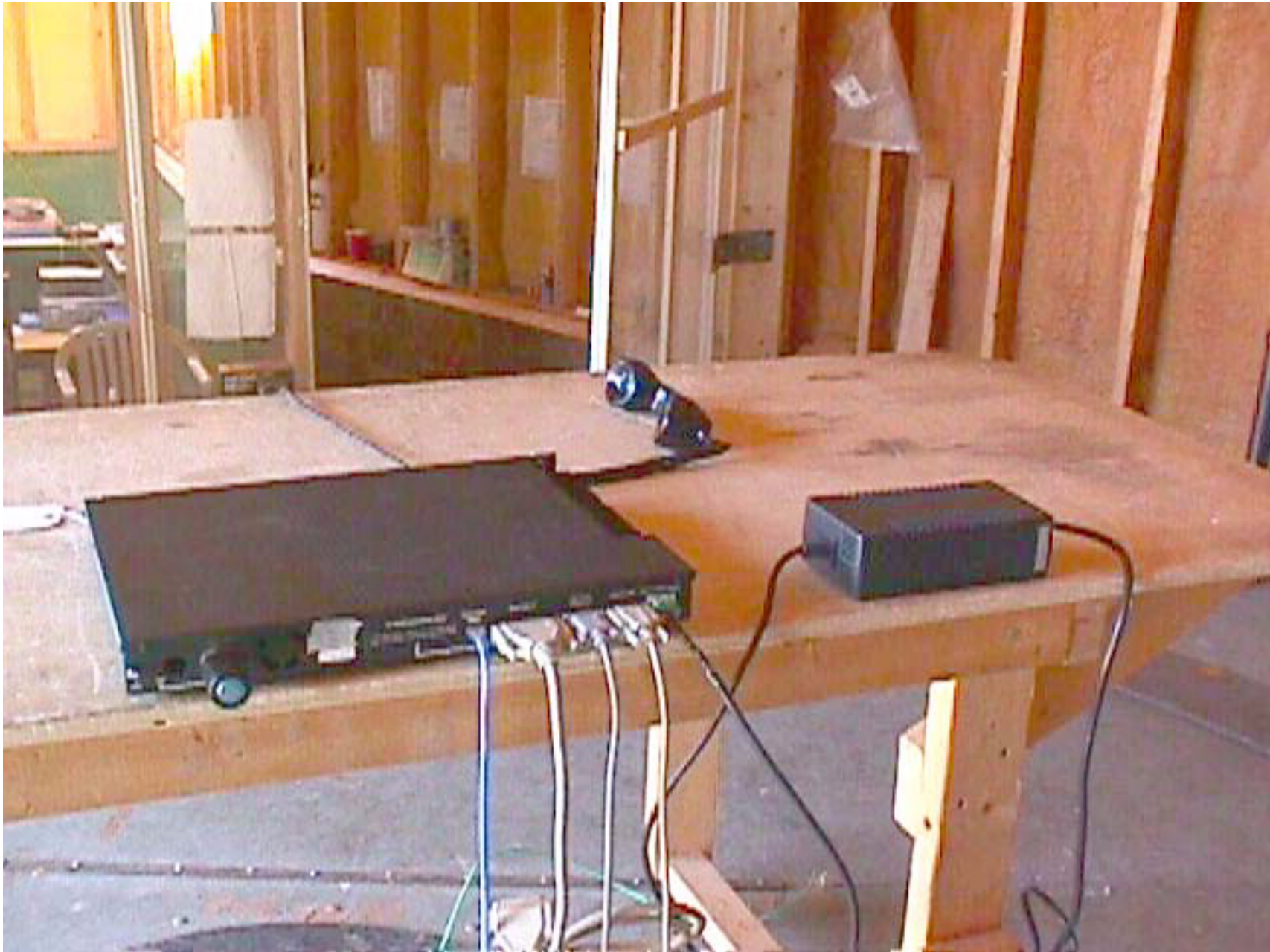
EXHIBIT 10 TEST SETUP PHOTOS RADIATED EMISSIONS AT 3 METERS DISTANCE FCC ID: E5M-LEDR400S
