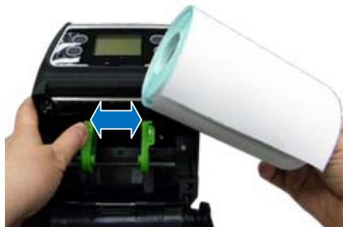
Pull the media holders apart far enough to fit the width of the label roll you are installing
