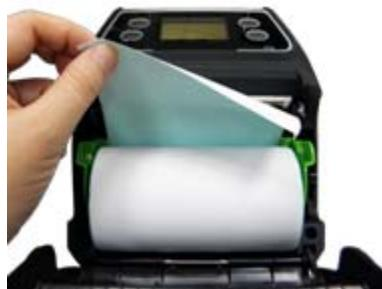
Place the roll, printing side face-out, between the media holders and insert hub into the core. Pull out enough paper above the printhead
