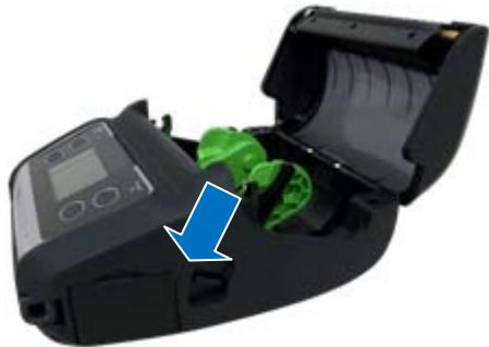
Open the printer media cover by pressing down on the media cover release latch.
