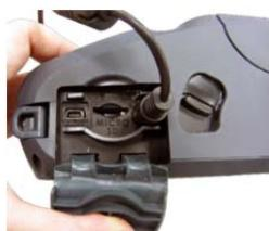
After installing the battery into the printer open the interface cover and plug the Charger power cord into the printer power jack
