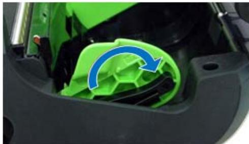
Push down each media holder lock lever to secure the media holders in place
