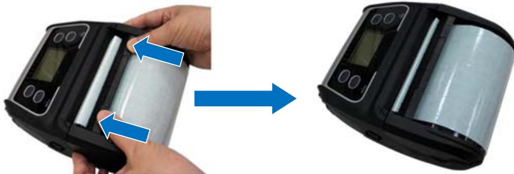
Push the label peel cover toward the front of the printer until it covers the plate roller
