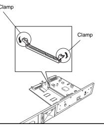
5 Remove the memory module from its package. Aligning the cutouts of the memory module with the matching keys of the socket, carefully plug the memory module into the memory socket until it clicks in place.
