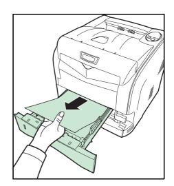
2 While pulling the green release lever, pull out the paper transfer unit.
