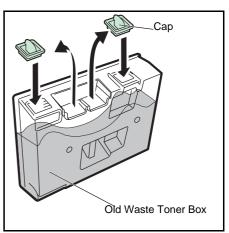
4 To prevent toner from spilling, put the old waste toner box in the plastic bag (contained in the toner kit) and discard it later according to the local code or regulations for waste disposal.
