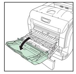
**3** Wipe away the paper dust on the registration roller (metal) using the lint free cloth.
