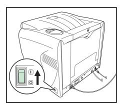
**IMPORTANT:** If you install the Toner Container and switch on the power, four indicators will start rapidly flashing. When the printer is first switched on after toner installation, there will be a delay of approximately 20 minutes before the printer is ready to print. Once the Ready indicator lights up, printer installation is complete.
