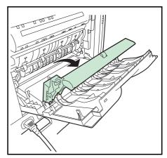
**3** Open the fuser cover and remove the jammed paper by pulling it out.
