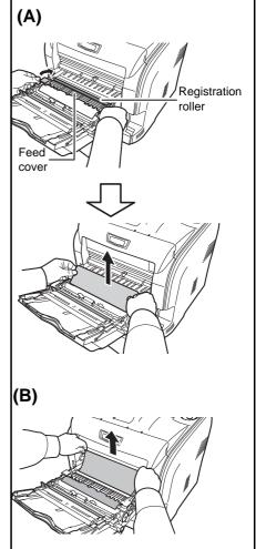
**4** Push the paper transfer unit back in completely. The printer warms up and resumes printing.
