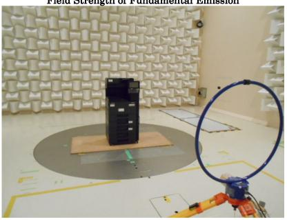
Radiated Spurious Emission (Below 30 MHz) Field Strength of Fundamental Emission
