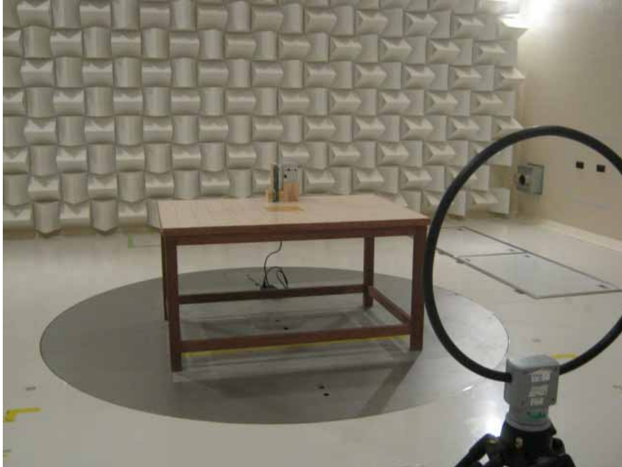
Angle 3, Front View (9kHz - 30MHz)
