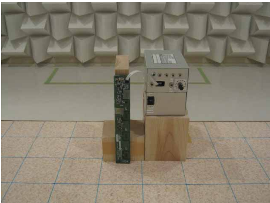
Angle 3, Close-up (30MHz – 1GHz)
