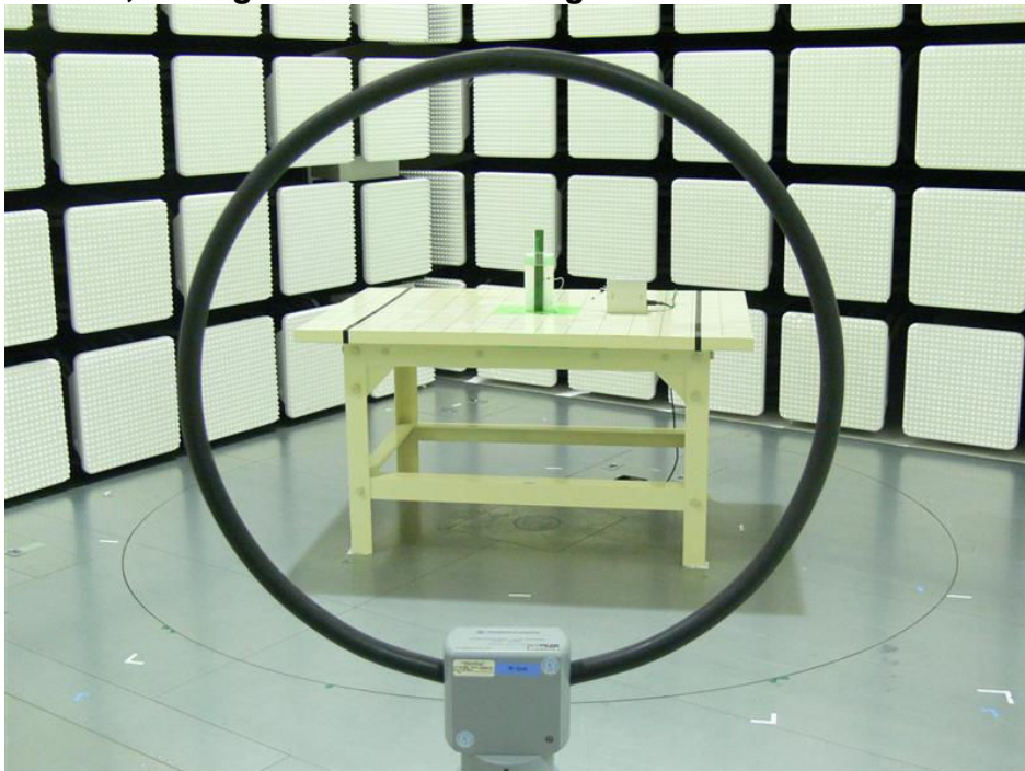
Photograph 7: Set-up for Radiated Emission of Transmitter including Loop Antenna, Configuration with Test Jig
