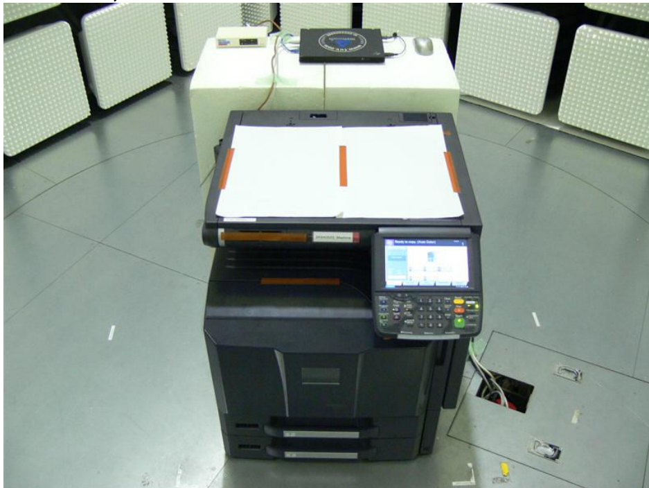
Photograph 11: Set-up for Radiated Emission of Transmitter, Configuration with Printer, Front View
