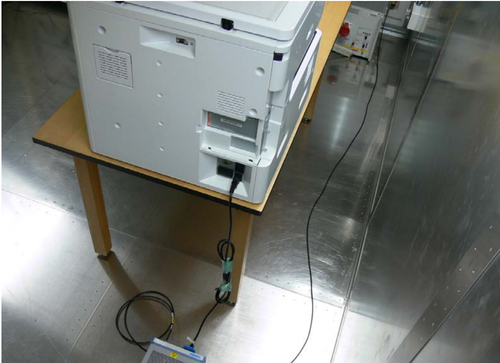
Photograph 4: Set-up for AC Power Line Conducted Emission of Transmitter, Rear View
