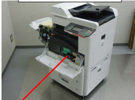
Front cover opens for replacing toner container.
