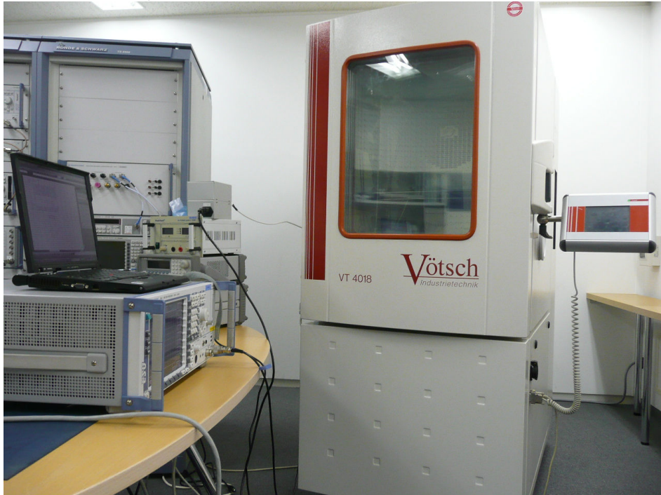
Photograph 2: Set-up for Antenna Port Conducted Emission Measurements, Overview
