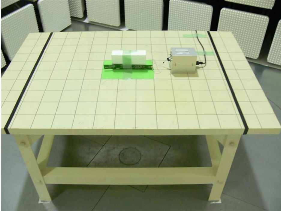
Photograph 8: Set-up for Radiated Emission of Transmitter, Configuration with Test Jig, Front View
