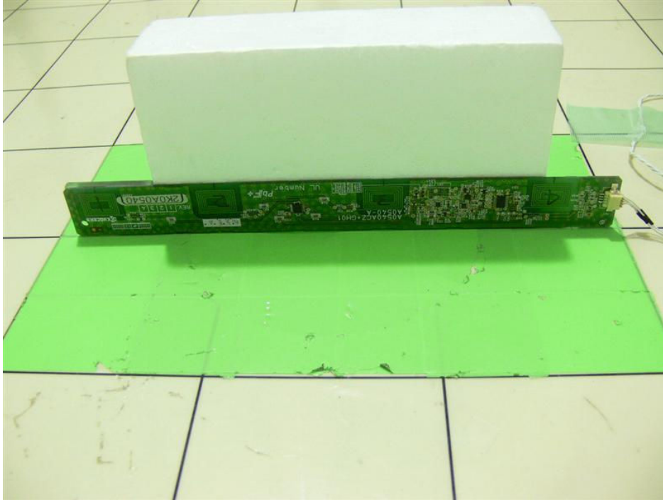
Photograph 6: Set-up for Radiated Emission, Configuration with Test Jig, EUT Orientation Z-Axis
