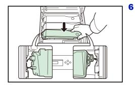
Set the new toner container in the printer as shown in the figure below.
