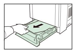
2 If paper is jammed in the paper cassette, open and close the front cover (the paper jam error will be reset).
