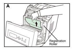
2 If paper is jammed as shown in **A**, remove the paper by pulling the center up. If paper is jammed as shown in **B**, remove the paper by pulling the edge.
