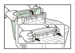
**2** Wipe away the paper dust on the registration roller and the paper ramp using the wiper cloth included in the toner kit.
