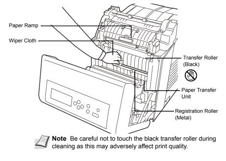
**3** Push the paper transfer unit back in completely.
