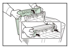
1 While pulling the green front cover release lever, pull out the front cover.
