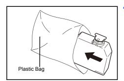
**4** To prevent toner from spilling, put the old waste toner box in the plastic bag (contained in the toner kit) and discard it later according to the local code or regulations for waste disposal.
