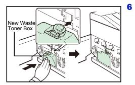
Insert the new waste toner box as shown in the figure below. When the box is set correctly, it will snap into place.
