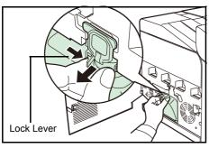
2 While holding the waste toner box, press the lock lever and then gently remove the waste toner box.
