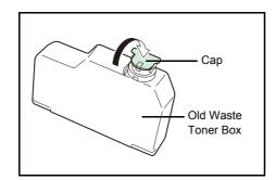
**3** Close the cap to the old waste toner box after removing the box from the printer.
