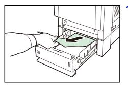
1 If the paper jams in the paper feeder, pull out the paper feeder and remove the jammed paper.
