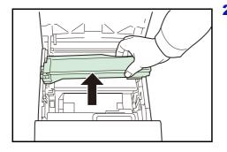
**2** Carefully remove the old toner container from the printer.
