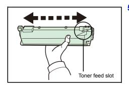
5 Shake the new toner container 5 or 6 times as shown in the figure in order to distribute the toner evenly inside the container. Do not press too firmly on the center of the toner container or touch the toner feed slot.
