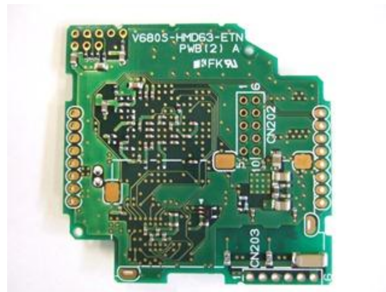
Fig. 29 V680S-HMD63-□ PCB(2) Side A without a shield plate
