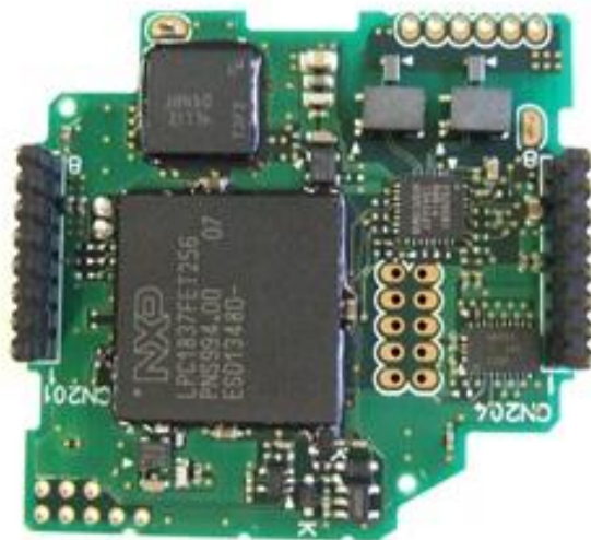
Fig. 30 V680S-HMD63-□ PCB(2) Side B
