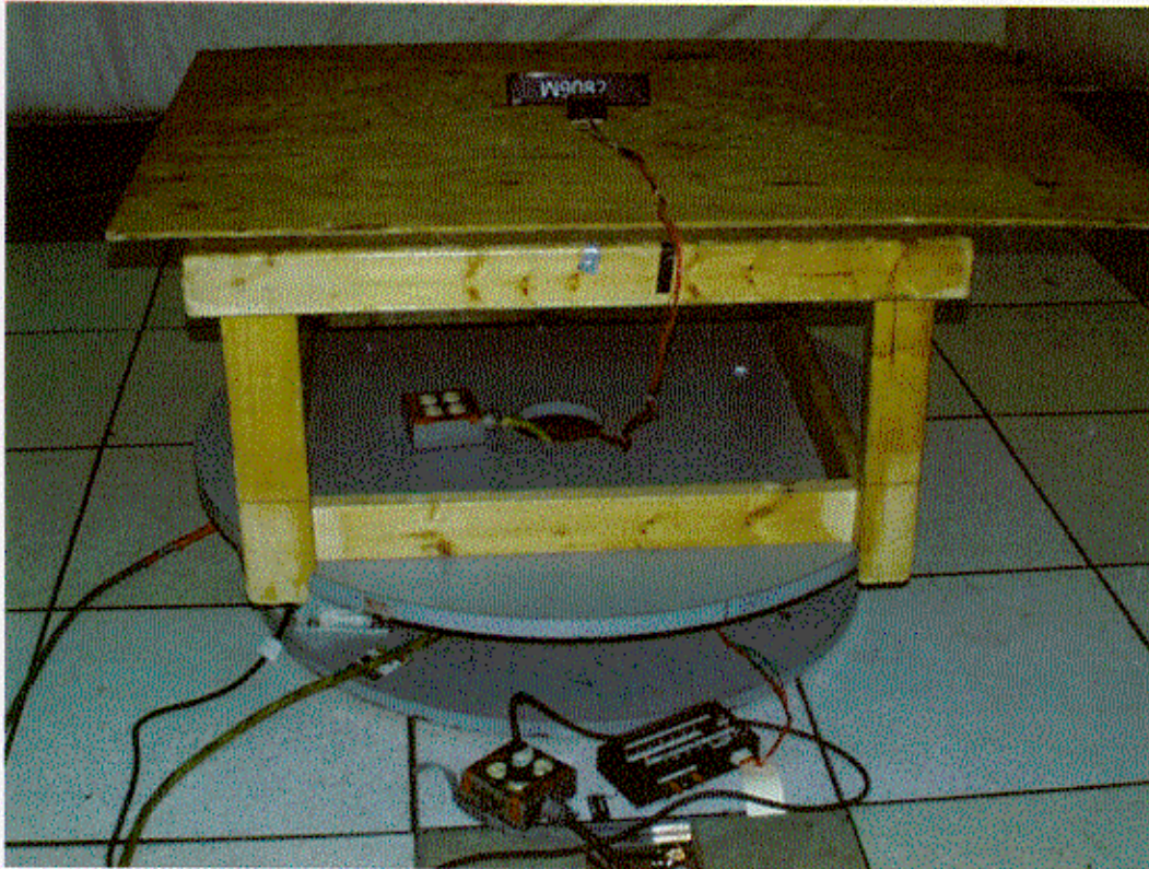
Test-setup photo(s): Radiated emission 30 MHz - 2000 MHz
