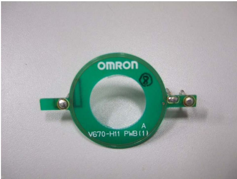
PWB (1) Side A of Antenna (V680-HS63)
