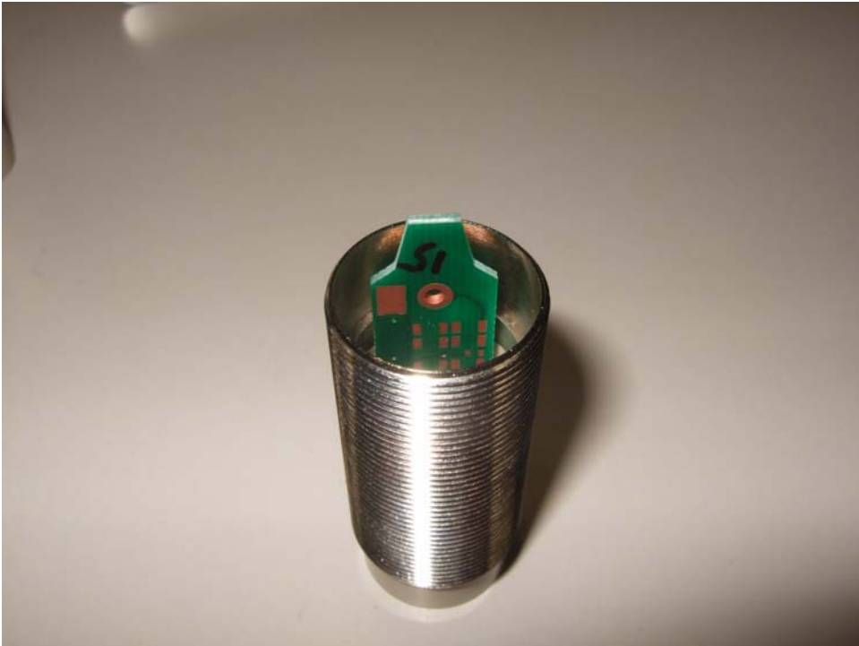
PWB(1) and PWB (2) in Case of Antenna (V680-HS52)
