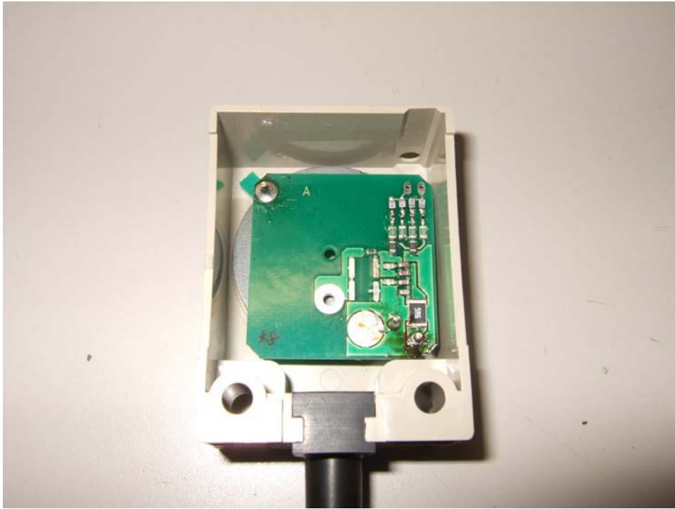
PWB(1) and PWB (2) in Case of Antenna (V680-HS63)
