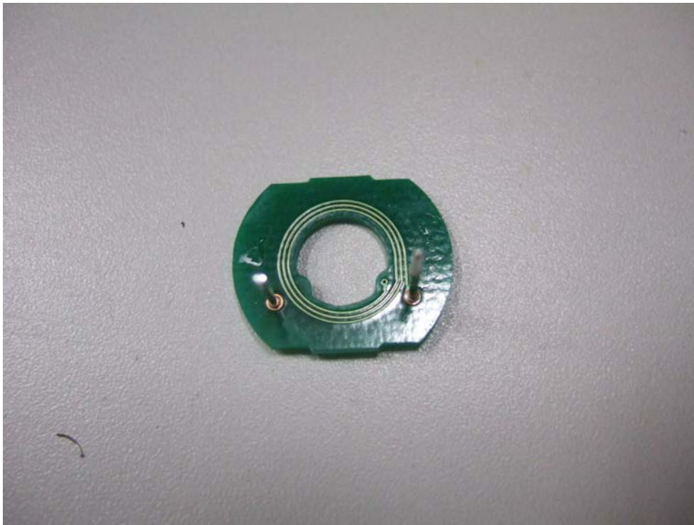
PWB (1) Side B of Antenna (V680-HS52)
