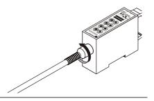
**2.** Pull the connector straight out of the port.
