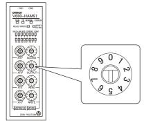
The position of the arrow in the figure is the direction in which the setting is made.
