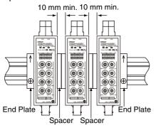
Use at least 2 OMRON DIN Track Spacers. (Each Spacer is 5 mm wide.)
