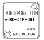
Mount the ID Tag to face the character printed surface with Antenna surface.
