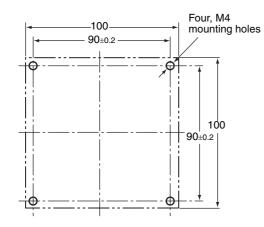
Use M4 screws and spring washers (in four places) for Antenna installation.
