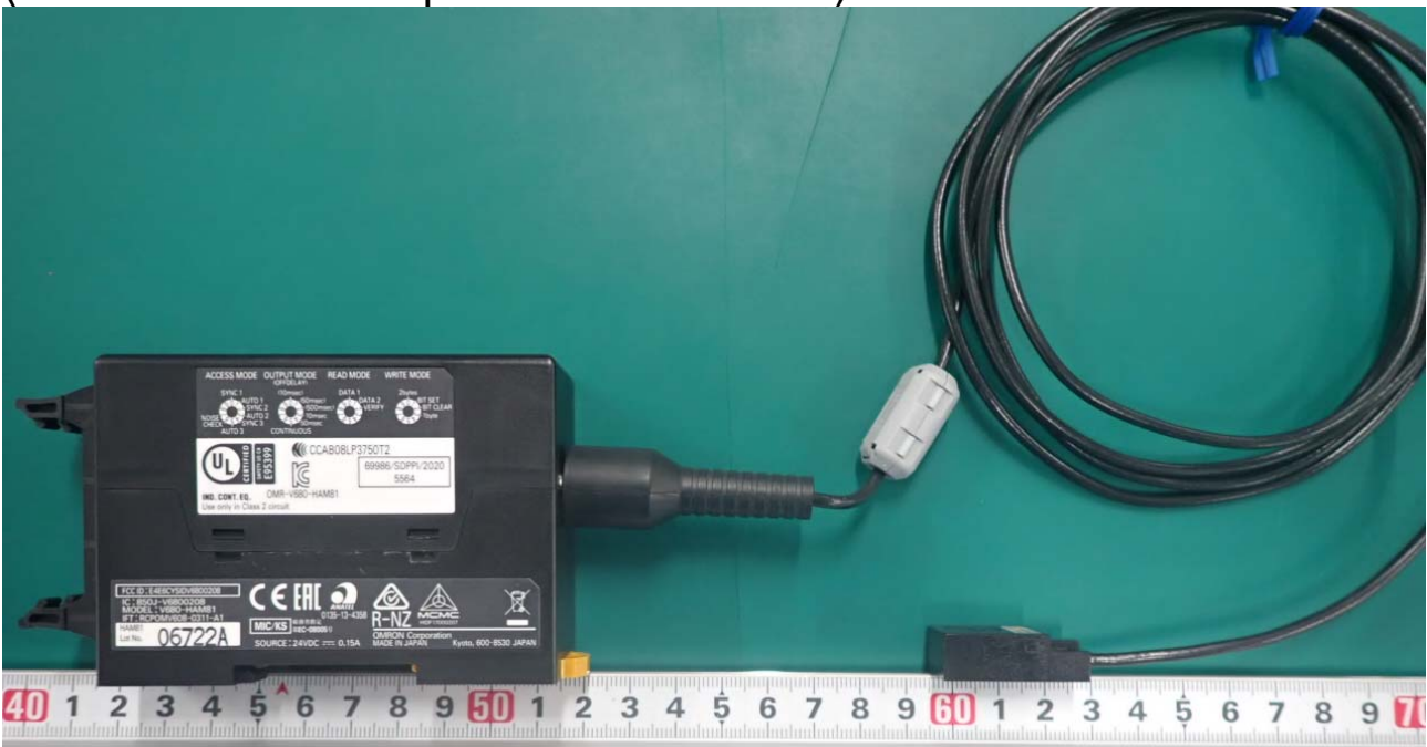
(connection with amplifier V680-HAM81)
