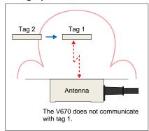
The V670 can communicate only with either of two specified tags (i.e., the tags with which the V670 previously communicated or a tags other than the previous ones.)
