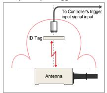
Whenever the V670 detects an input signal rise, the V670 will check the existence of the corresponding tag repeatedly and communicate with the tag. An error will result if the tag cannot be detected.
