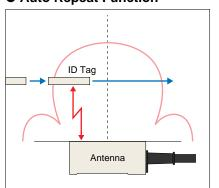
The V670 is in repeated communications with tags coming into the communications range. The V670 does not, however, communicate with the same tag more than once.
