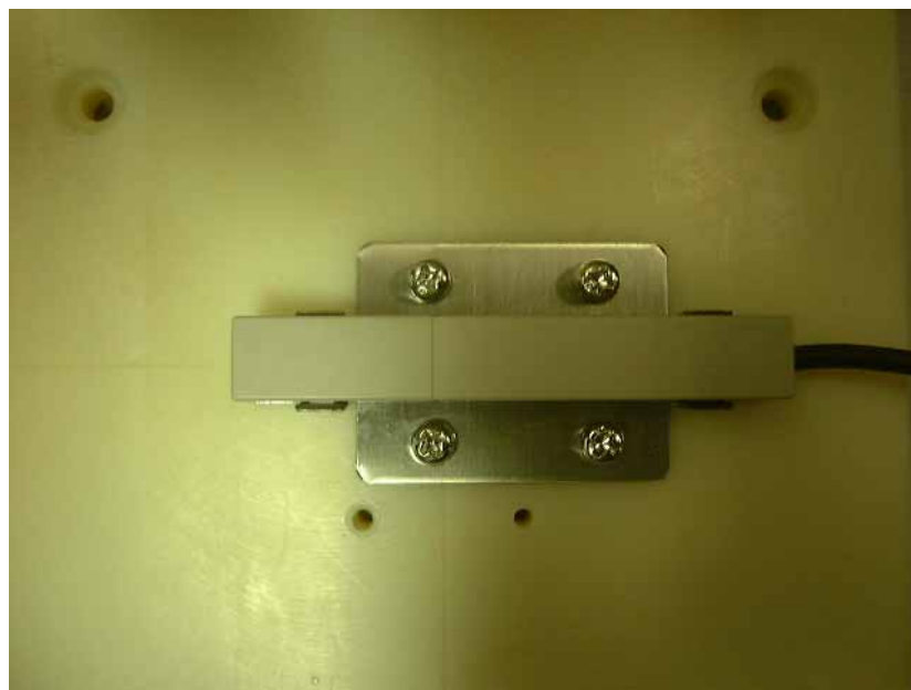
Head of Antenna: CIDRW Head V640-HS62 (-X)
