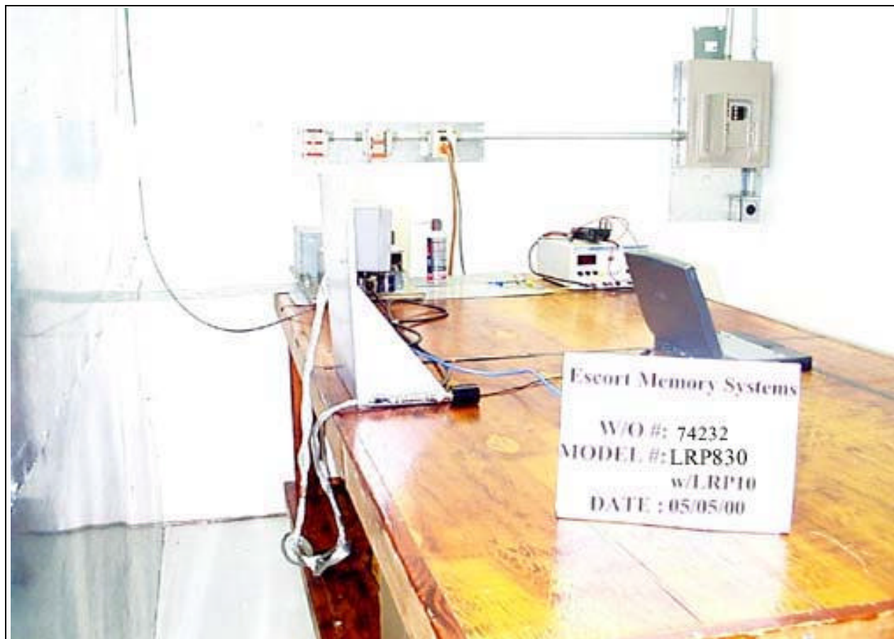
Conducted Emissions - Back View with DC Load
