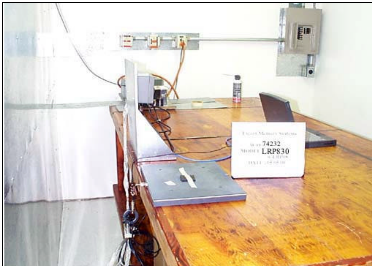
Conducted Emissions - Back View with Antenna 08
