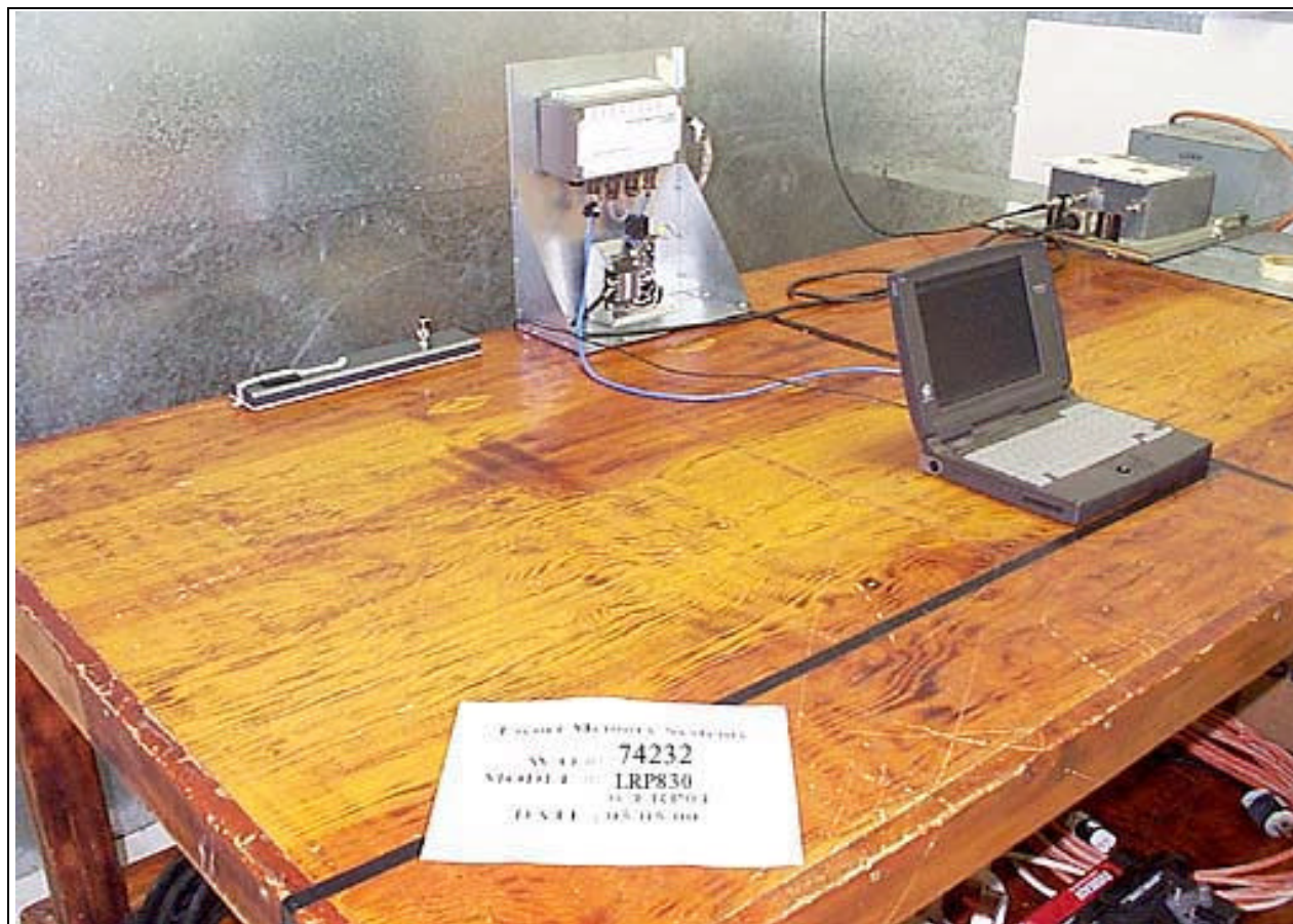
Conducted Emissions - Front View with Antenna 04
