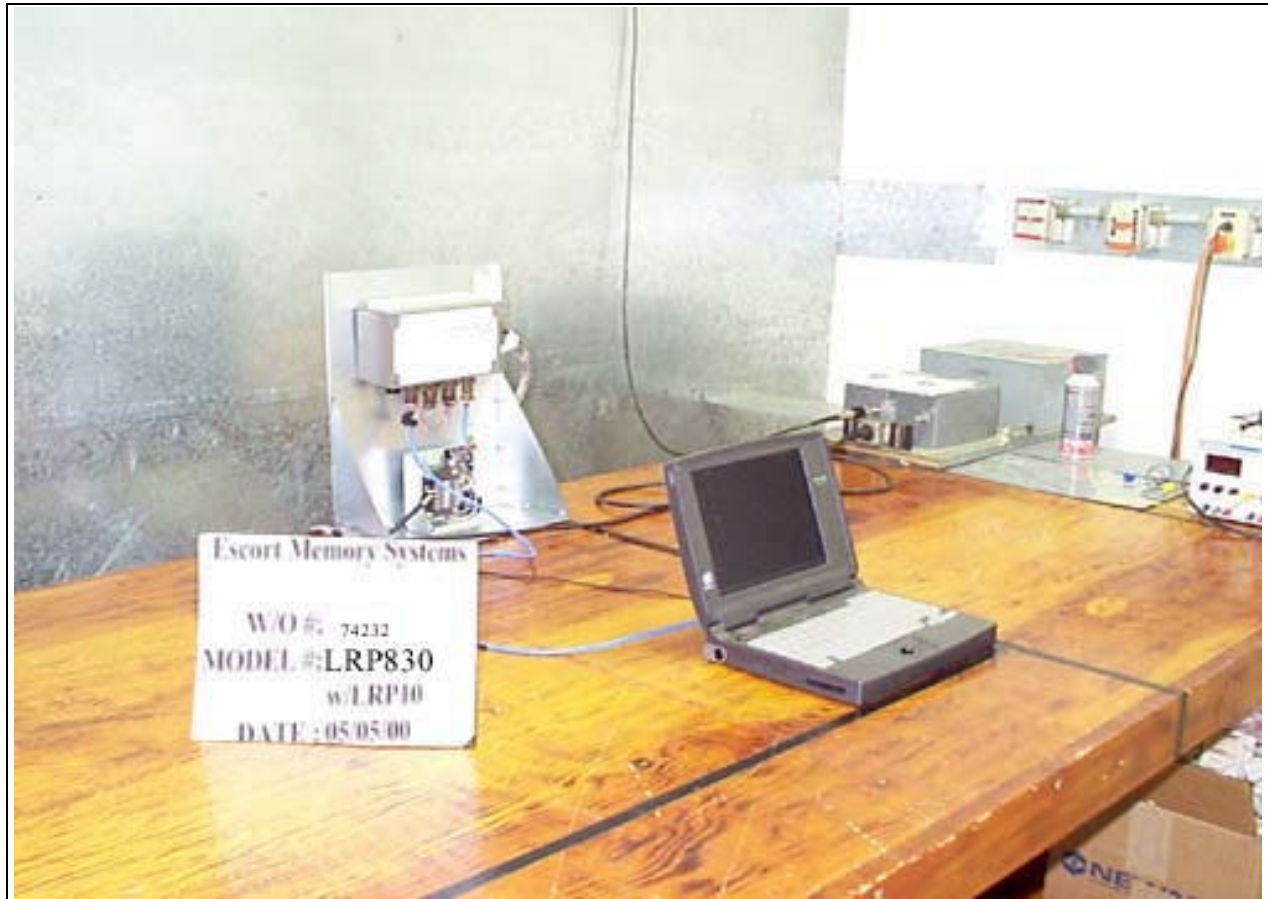
Conducted Emissions - Front View with DC Load
