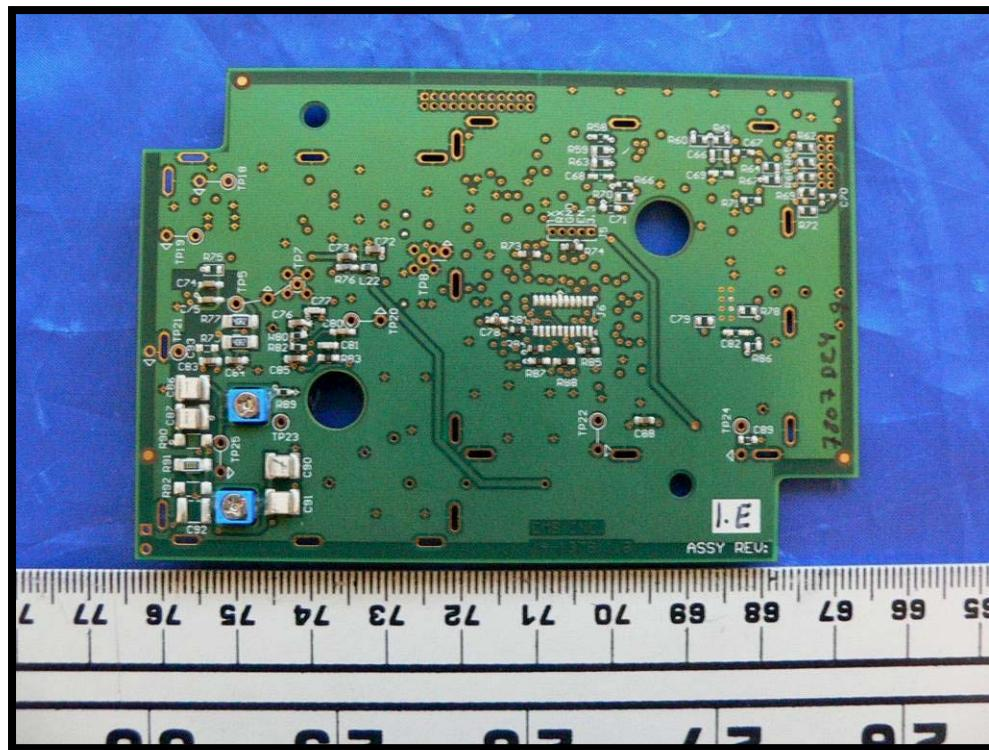
**11.7 EUT – Sub - Board Component View (C1007 – 232/485/USB – 01)**
