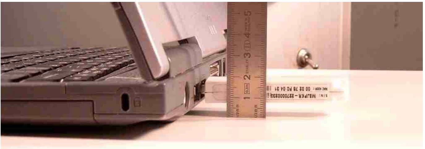
Photo 5 : Side view. Offset dongle to base = 8 mm
