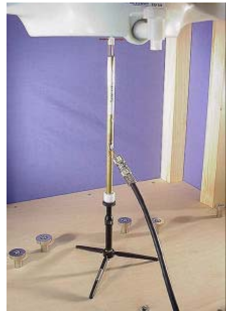
2450MHz System Check Setup Photograph
