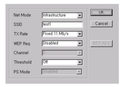
**Configuration Change** screen allows you to set the parameters as explained below.
