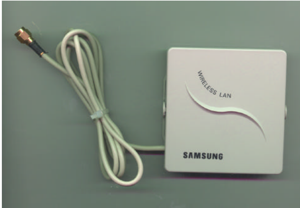
Figure 19: ISA Antenna (Front)
