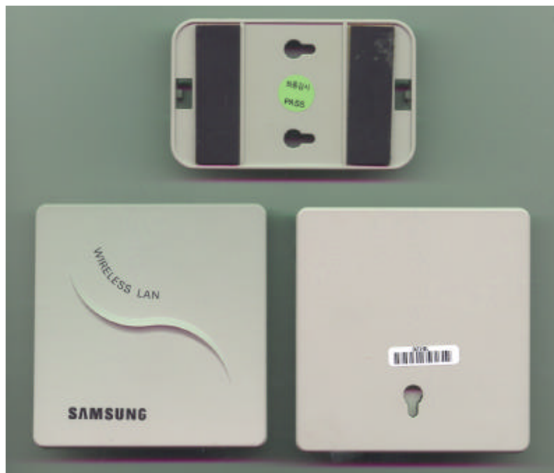
Figure 22: ISA Antenna Outside Bracket & Cover
