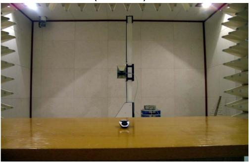
Final Measurements were EUT at 3m test range using Logbicon Super Antenna (ARA, LBP-2520/A) and horn antenna. (Electro-Metrics RGA-60)
