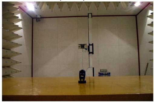
Final Measurements were EUT at 3m test range using Logbicon Super Antenna (ARA, LBP-2520/A) and horn antenna. (Electro-Metrics RGA-60)
