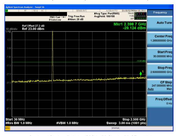
■ Conducted Spurious Emission (QPSK – RB Size 25, RB Offset 12)-2
