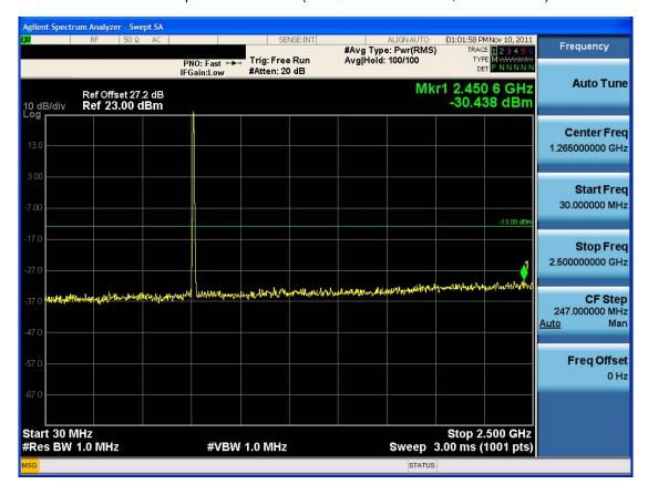
■ Conducted Spurious Emission (16-QAM – RB Size 25, RB Offset 12)-2
