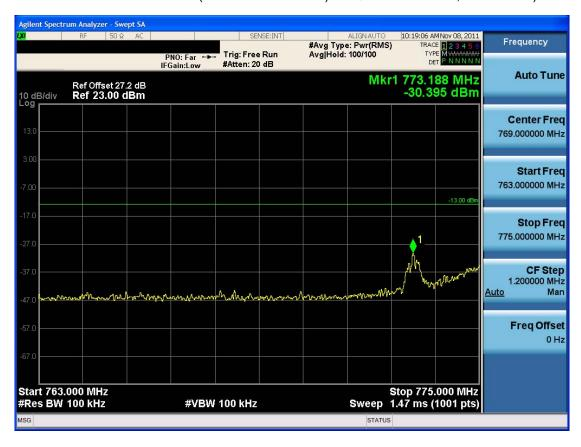
■ Low Emission Mask (763 MHz – 775 MHz) 16-QAM –RB Size 50
