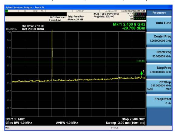
■ Conducted Spurious Emission (16-QAM – RB Size 1, RB Offset 0)-2
