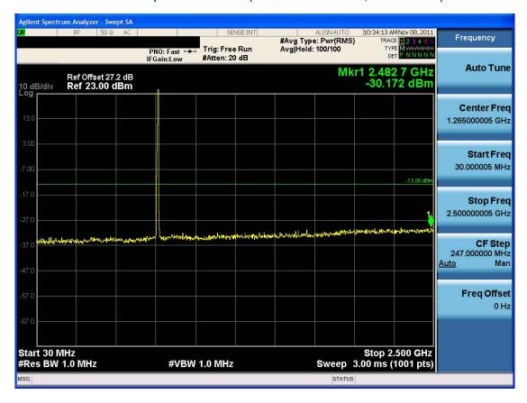
■ Conducted Spurious Emission (16-QAM – RB Size 1, RB Offset 49)-2
