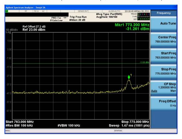
■ Low Emission Mask (763 MHz – 775 MHz) QPSK –RB Size 50
