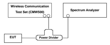
(Configuration of conducted Emission measurement) Test Procedure
