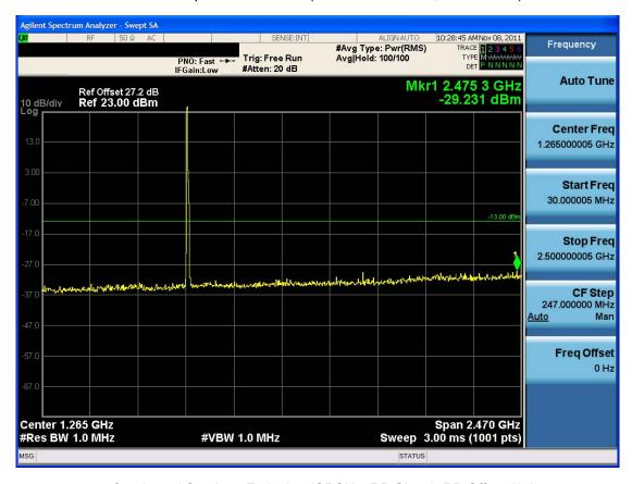
■ Conducted Spurious Emission (QPSK – RB Size 1, RB Offset 0)-2
