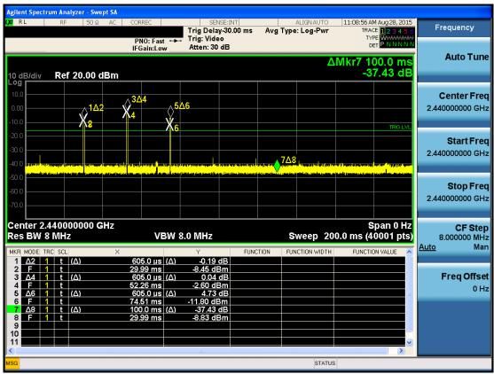
Note : Measure Duty Cycle = T / 100 ms ( T = sum of the individual on-time in 100 ms ) = ( 0.605 ms + 0.605 ms + 0.605 ms ) / 100 ms = 1.815 % Declared worst Duty Cycle = 3.9 %
