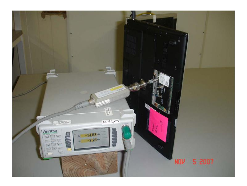
Maximum Peak Output Power Measurement Setup
