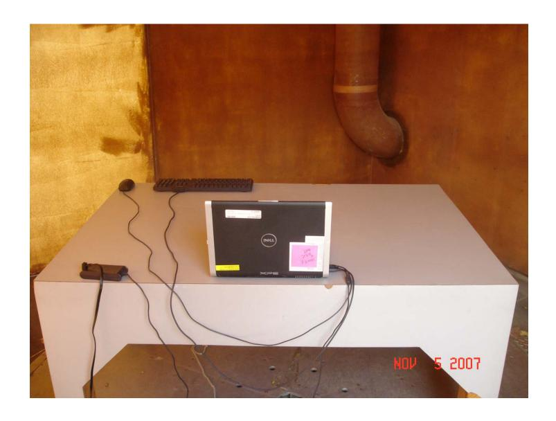
Radiated Emissions Measurement (Rear View – Hawke Platform) Setup
