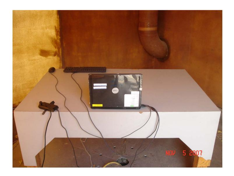
Radiated Emissions Measurement (Rear View – Spears Platform) Setup
