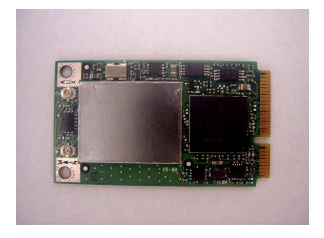
Top View "Insulation removed"
