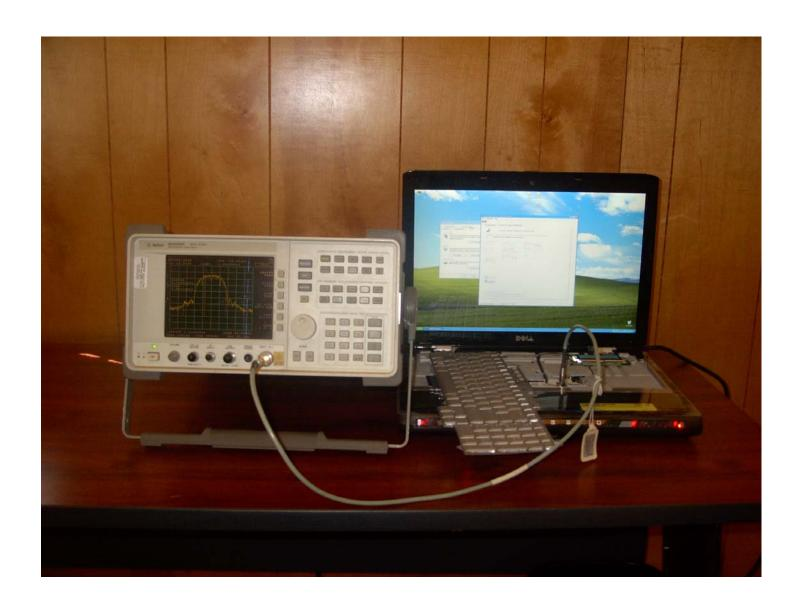
Conducted Emissions at Antenna Terminal Setup
