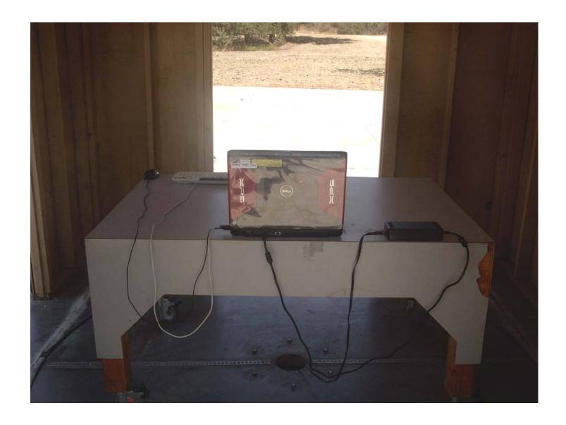
Radiated Emissions Measurement (Rear View) Setup
