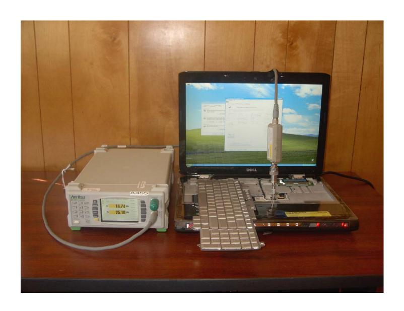
Maximum Peak Output Power Measurement Setup
