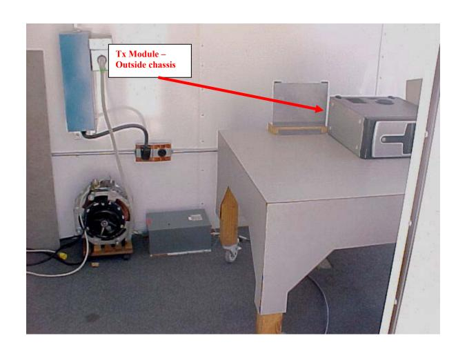
AC Conducted Emissions Measurement (Front View) Setup
