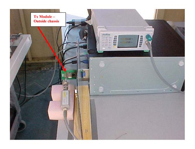
Maximum Peak Output Power Measurement Setup
