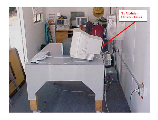
AC Conducted Emissions Measurement (Rear View) Setup
