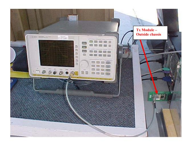
Conducted Emissions at Antenna Terminal Setup
